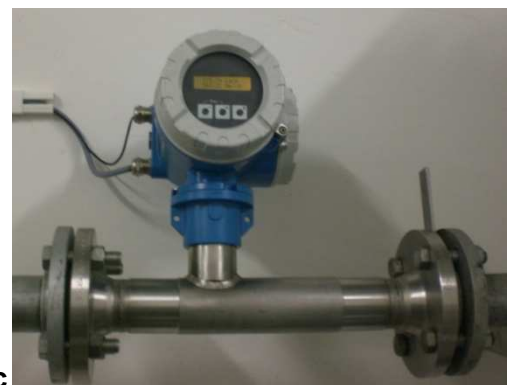
Figure 2-5 a) inductive sensor for rotational speed measurement [PICOTURN], b) Piezoresistive sensors for static pressure measurement [Sensor technics] c) Proline t-mass 65 flow meter.
