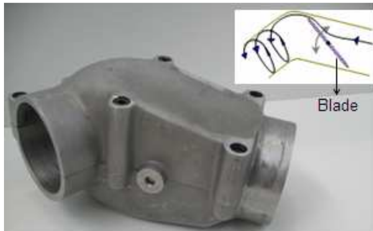
Figure 4-8 Tested one blade radial guide vane system [RGVs]
