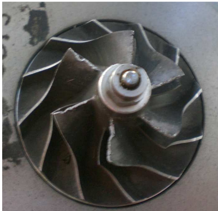
Figure C-10 damaged impeller leading edge due to non filtered air at the compressor inlet
