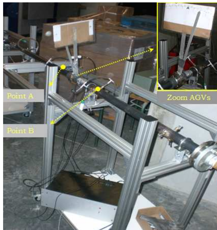
Figure 4-12 AGVs pressure loss test bench
