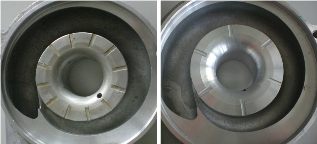
Figure 4-66 tested J grooves configurations. GR1 to the left and GR2 to the right
