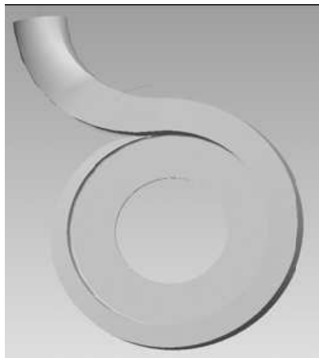
Figure 1-20 Volute modifications with exit turning about the axis (67)
