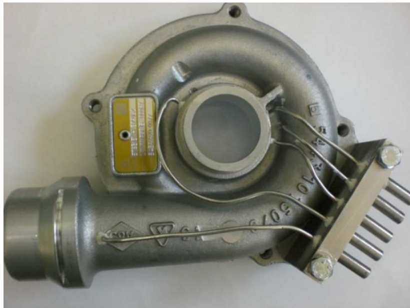
Figure 3-8 Pressure transducers installation
