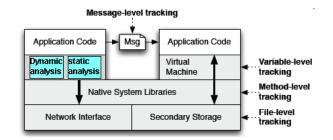
Figure 6.6: TaintDroid Approach. Our Approach is implemented in Dalvik virtual machine (Blue)
