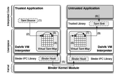
Figure 6.7: TaintDroid architecture [5]
