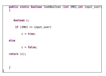
Figure 6.15: LeakBoolean function source code
