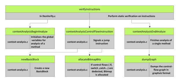
Figure 6.12: Calling sequence of functions added.
