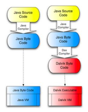
Figure 6.2: Difference between JVM and DVM [142].
