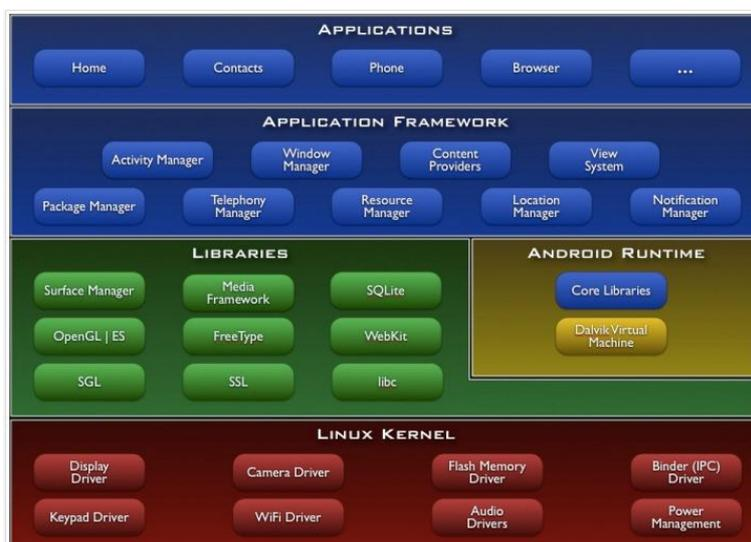
Figure 6.1: Android operating system architecture.
