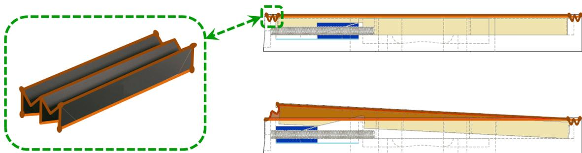
Figure 4.21 – the elastic micro-membrane employed for the actuation system components sealing
