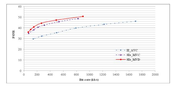
Figure 4.32: Performance of proposed compression method (labeled 'SIs\_MVD'), MVC-based method (labeled 'SIs\_MVC') and baseline H.264/AVC method (labeled 'II\_AVC')
