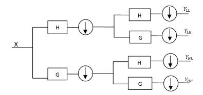
Figure 4.21: 2D-DWT decomposition
