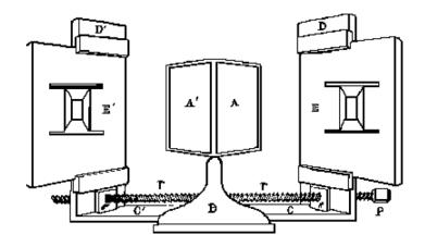
Figure 1.1: The Wheatstone stereoscope, mirrors A' and A are set at an angle in order to reflect the left and right eye drawings (E' and E) towards the viewer's eyes
