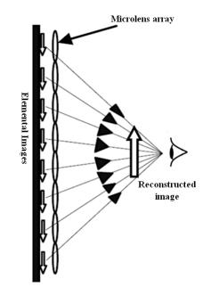
Figure 5.2: Principle of view-based CIIR
