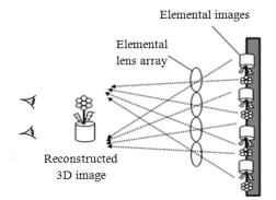
Figure 5.1: Optical setup for displaying 3D scene in integral imaging system
