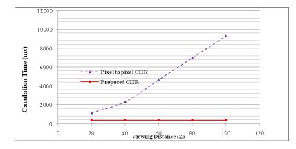
Figure 5.20: Computation cost of pixel-to-pixel and parallel-group projection CIIR for the 3D scene 'cube'
