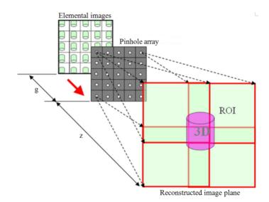
Figure 5.5: Principle of plane-based CIIR
