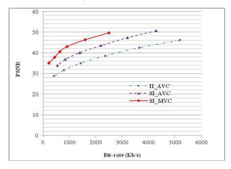
Figure 4.26: Performance of MVC compression scheme for SIs, AVC scheme for SIs and baseline AVC scheme for integral images sequence
