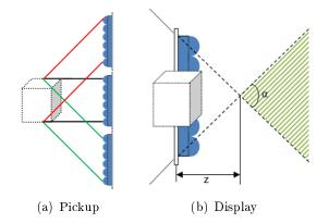
Figure 3.11: Pickup and display process of depth controlling CIIG method
