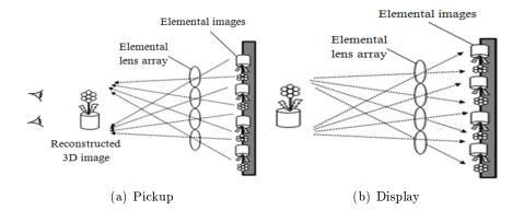
Figure 3.1: Optical setup of integral imaging system
