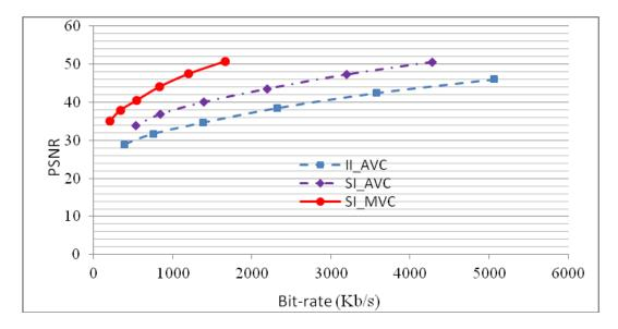
Figure 4.29: Performance of MVC compression scheme for SIs, AVC scheme for SIs and baseline AVC scheme for integral images sequence
