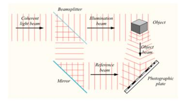
Figure 2.12: Hologram recording
