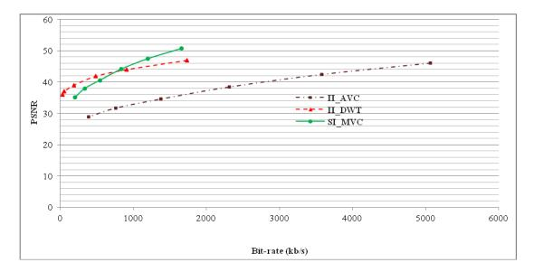
Figure 4.36: Performance of proposed compression method (labeled 'SIs\_MVD'), MVC-based method (labeled 'SIs\_MVC') and baseline H.264/AVC method (labeled 'II\_AVC')
