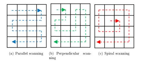
Figure 4.6: Three different mode for scanning elemental images in an II
