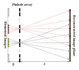
Figure 5.8: Reconstruction principle of pixel-to-pixel mapping CIIR method
