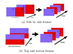
Figure 2.8: Frame compatible transmission format
