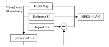
Figure 4.18: Flow chart of proposed compression method
