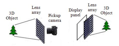
Figure 2.11: Optical setup for generating (left) and displaying (right) 3D scene in integral imaging system
