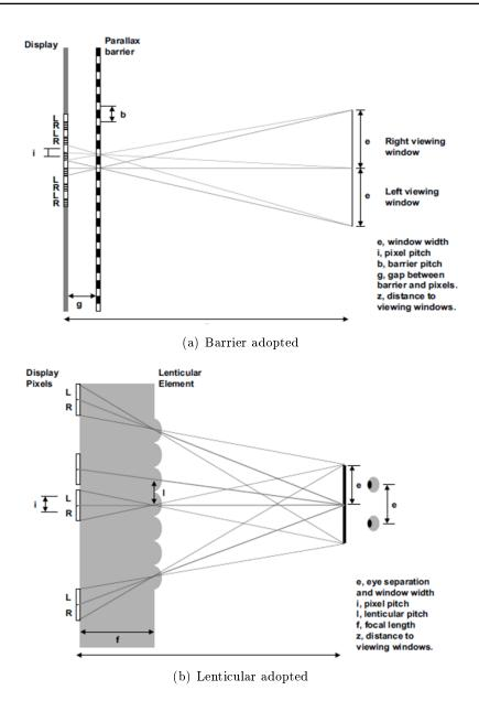
Figure 2.9: The principle of auto-stereoscopic display
