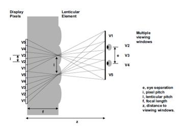
Figure 2.10: The principle of a multi-view auto-stereoscopic display
