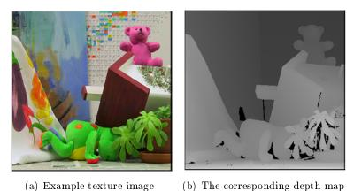
Figure 2.5: Example of this video plus depth representation format
