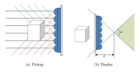
Figure 3.10: Pickup and display process of traditional CIIG method
