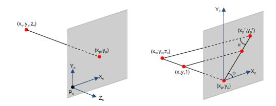
Figure 4.19: Mapping a 3D point to 2D clip plane by orthographic (left) and oblique (right) projection
