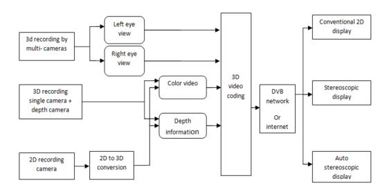
Figure 2.2: Structure of Complete 3DTV Processing Chain
