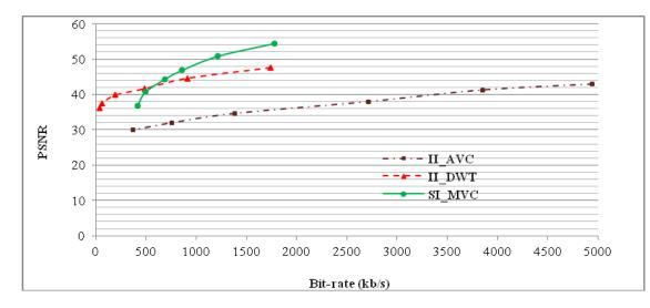
Figure 4.34: Performance of proposed compression method (labeled 'SIs\_MVD'), MVC-based method (labeled 'SIs\_MVC') and baseline H.264/AVC method (labeled 'II\_AVC')
