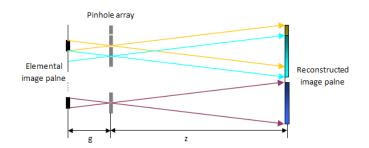
Figure 5.7: Reconstruction principle of traditional CIIR method
