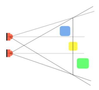
Figure 2.3: Parallel cameras model
