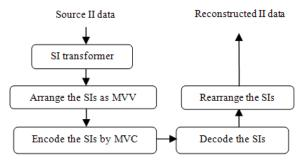
Figure 4.13: Flow chart of the proposed integral images compression system
