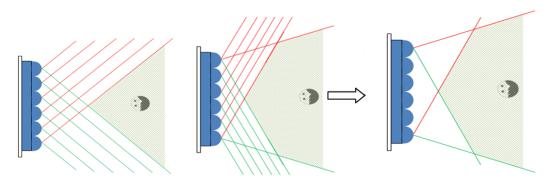
(a) Traditional CIIG generated (b) Initial II with large viewing (c) Proposed CIIG generated II with small viewing range range II with large viewing range
