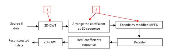
Figure 4.20: Flow chart of the compression scheme
