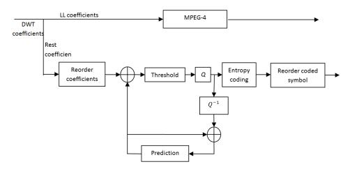
Figure 4.23: Hybrid MPEG-4 based method
