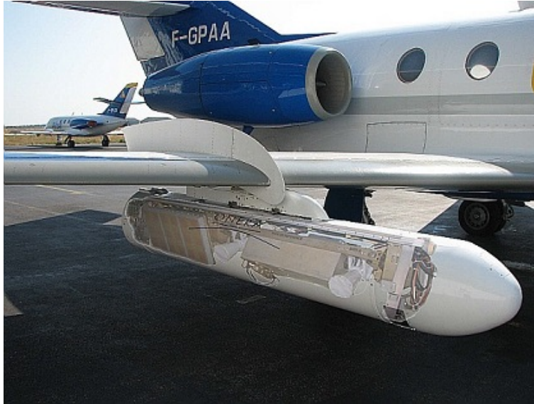
FIGURE 1.1: Right pod of the SETHI facility of ONERA that carries a radar antenna
