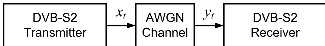
Figure 6.1: DVB-S2 transmission chain
