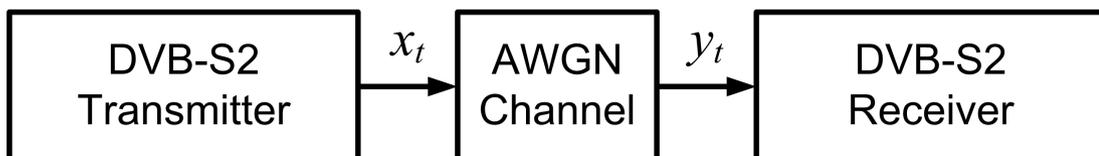
Figure 6.1: DVB-S2 transmission chain
