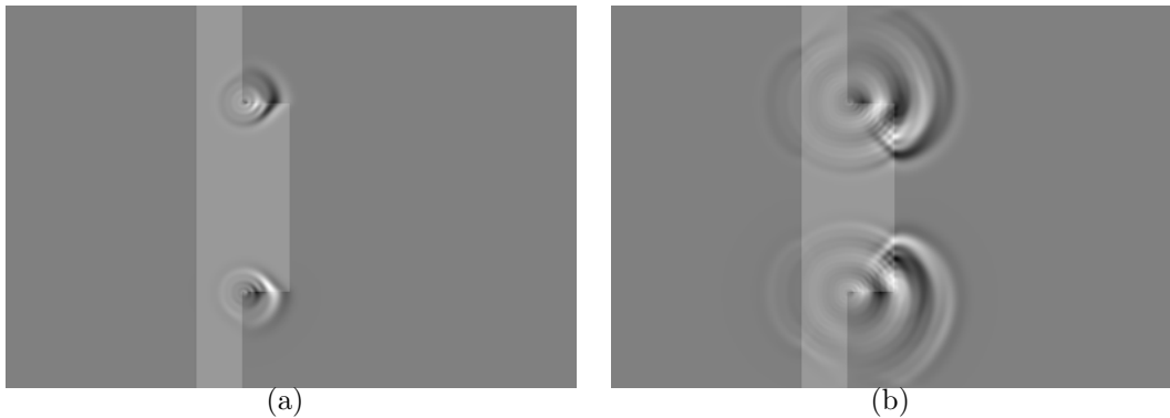
Figure 4.2 — The state of H_z obtained by the FDTD simulation (MEEP): (a) after 4.5 optical cycles, and (b) after 6 optical cycles.
