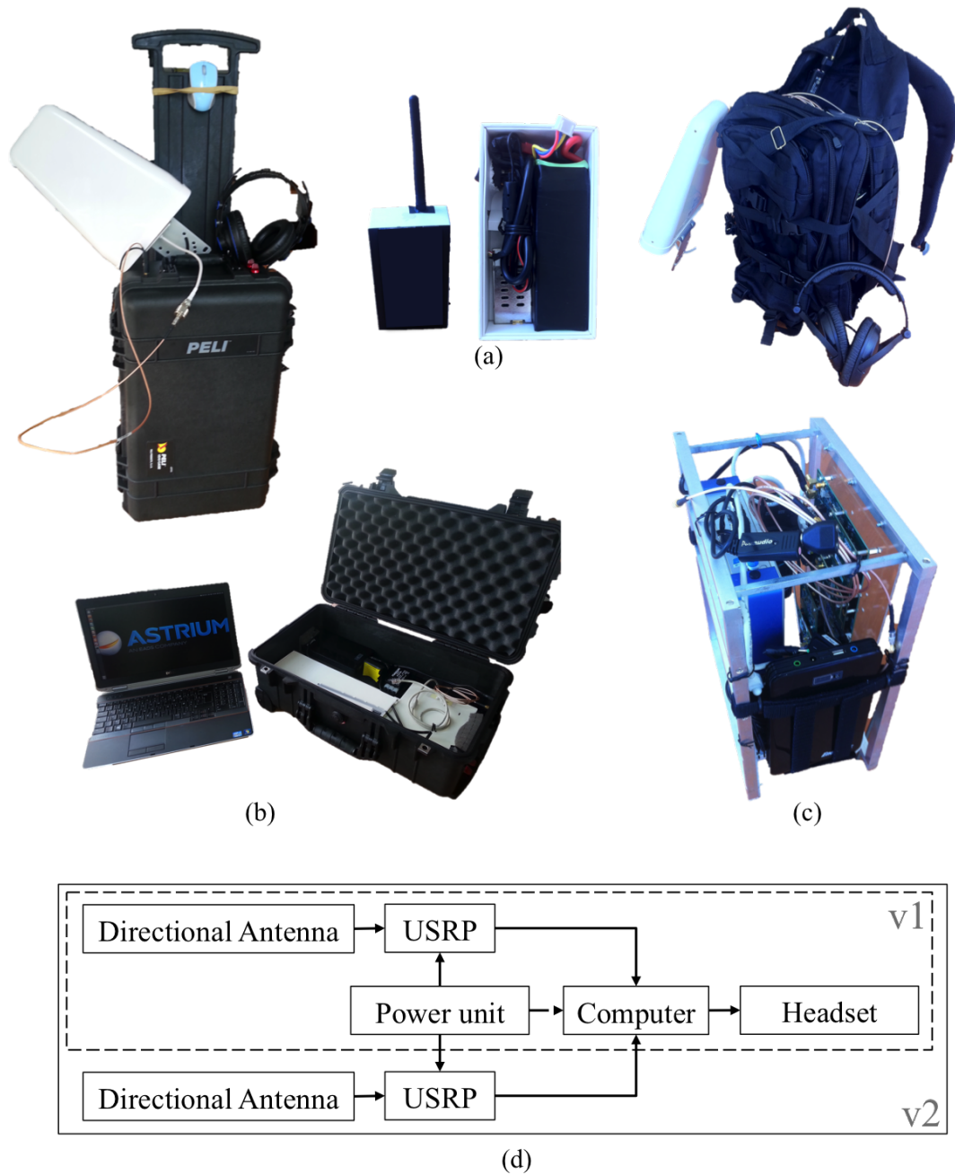
Figure 11.7: Illustration of the RF emitter (a) and the PP v1 (b) and v2 (c). RF emitter sized 7.5\text{cm} \times 13\text{cm} \times 4\text{cm} ( W \times H \times D , in cm) and weighted 300 g. PP v1, handle folded, sized 34\text{cm} \times 54\text{cm} \times 23\text{cm} and weighted 16 kg. PP v2 aluminum structure sized 28\text{cm} \times 35\text{cm} \times 17\text{cm} for a total backpacked size of 31\text{cm} \times 46\text{cm} \times 23\text{cm} and weighting 8 kg. (d) Simplified block diagram of both v1 and v2 prototypes.
