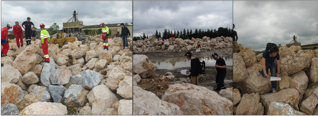
Figure 11.8: Illustrations of the tests sessions with the SDIS. Comparison of search performance between DF_1 , geo-stereophone and dogs. Victims were trapped under the rubbles, equipped with the RF transmitter pictured Figure 11.7a.
