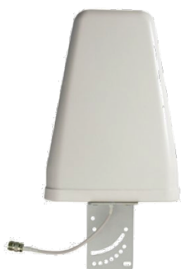
Figure 11.2: Illustration and specifications of the Yagi-Uda directional antenna used for the DF prototype. Its radiation pattern is a cardioid defined by Apertures V and H. For example, according to the figures of Aperture GSM900 H, the antenna gain for a GSM900 source emitting above the pictured antenna would be of 8.2 dBi and would be decreased by 3 dB if the source was shifted left or right from 90^\circ/2 = 45^\circ .
