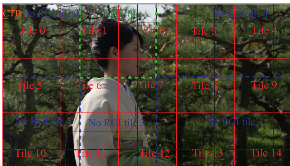
Figure 6.9: Tile concept in the HEVC standard composed of 15 tiles (red rectangles)
