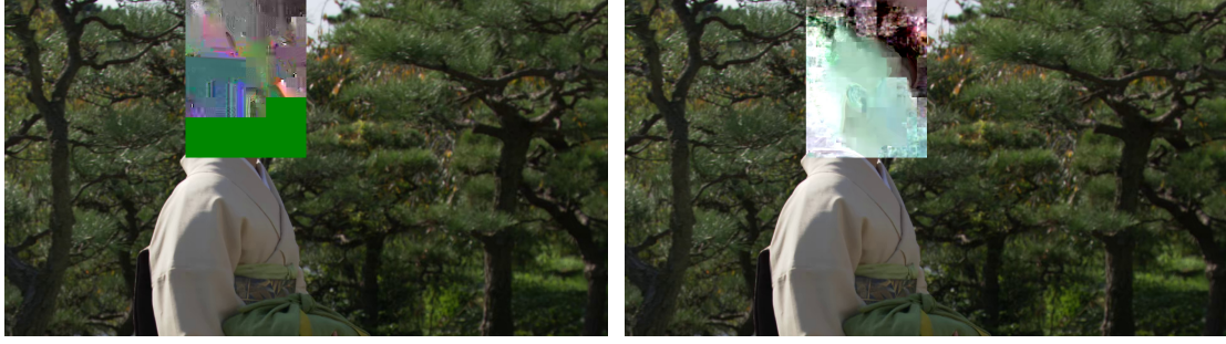
(a) TNE-HEVC PSNR1=10.95, PSNR2=42.07, PSNR3= 21.15(dB) (b) TSE-HEVC PSNR1=7.78, PSNR2=42.07, PSNR3=18.01 (dB)
