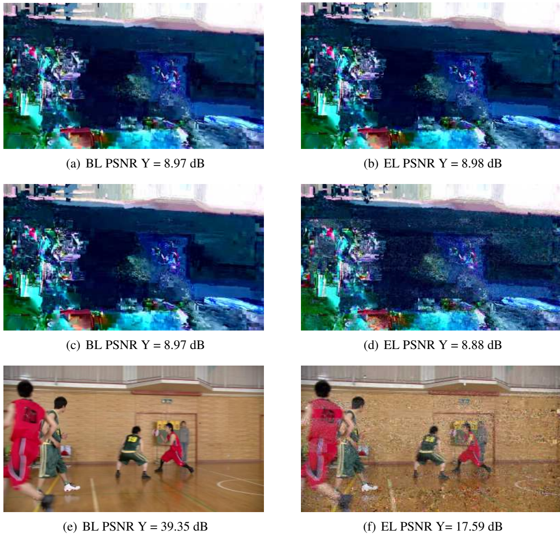
Figure 6.5: Visual quality of frame #9 of the BasketballDrive video sequence in SNR scalability configuration (a) (b) SE-SHVC-BL, (c) (d) SE-SHVC-ALL and (e) (f) SE-SHVC-EL)
