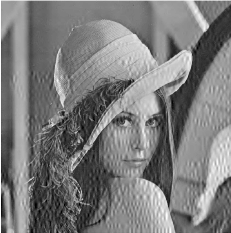
FIG. 1. – JPEG 2000 image reconstruction including resilient mechanisms after a burst error of thirty consecutive bytes starting at byte 0xD9C.
