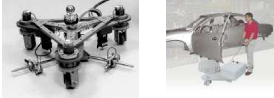
Figure 1.5: Scooter cobot: virtual paths are implemented thanks to the computer-controlled steering of the three wheels, in order to reduce inertia effects in direction changes.
