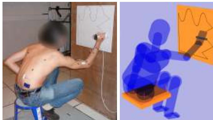
Figure 4.9: Left: A human subject performs the task while his motion and interaction forces are recorded. Right: The motion is replayed with the virtual manikin and the LQP controller.
