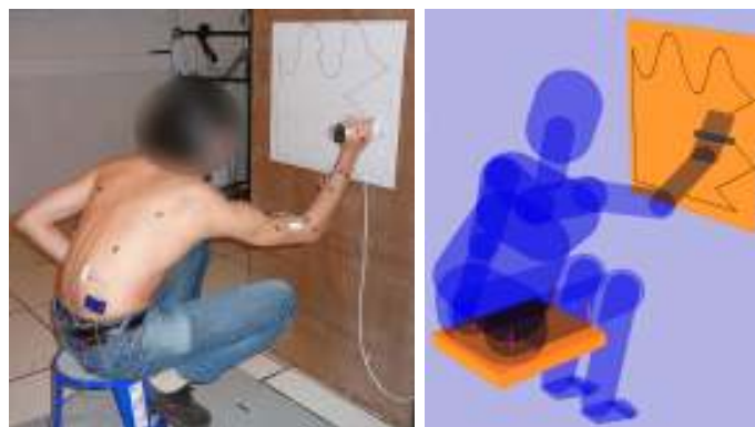
Figure 4.9: Left: A human subject performs the task while his motion and interaction forces are recorded. Right: The motion is replayed with the virtual manikin and the LQP controller.
