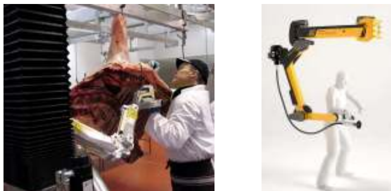
Figure 1.6: Collaborative robots providing strength amplification. Left: HookAssist (Kinea Design) for beef boning. Right: Cobot 7A.15 (RB3D, CEA-LIST, CETIM) for tire retreading or machining.
