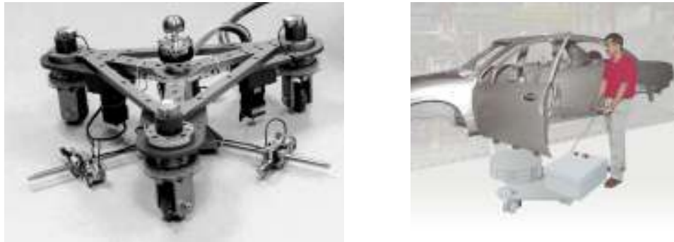
Figure 1.5: Scooter cobot: virtual paths are implemented thanks to the computer-controlled steering of the three wheels, in order to reduce inertia effects in direction changes.
