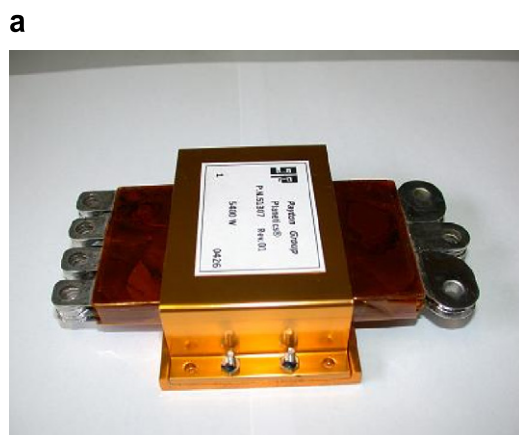
Fig. 24. High frequency planar transformer used for the design of the power converter. (a) 5400 W–50 kHz planar transformer from Payton company, (b) Characteristics of the high frequency planar transformer.
