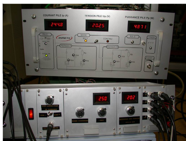
Fig. 5. Front panel of the active load with control-command set.
