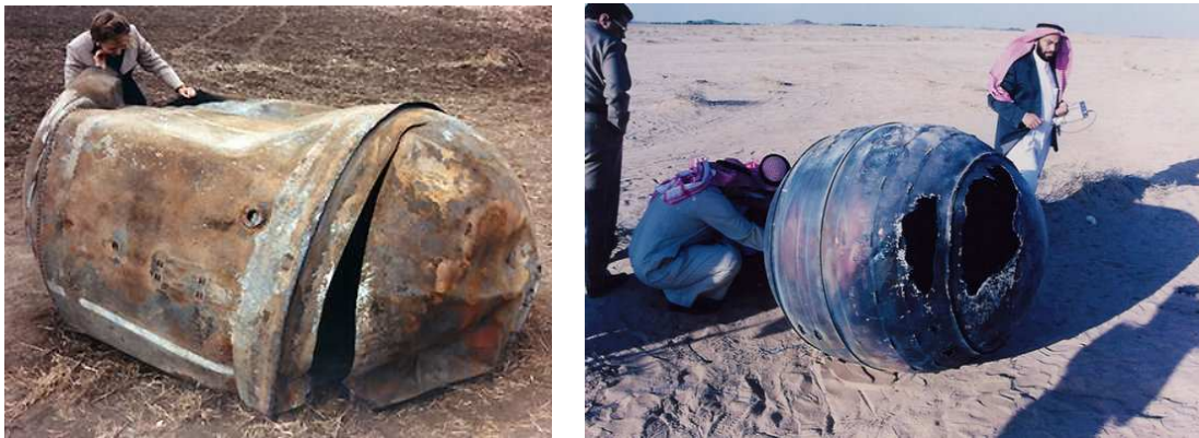
Figure 1.3: Large objects re-entries: the second-stage propellant tank of a Delta II launch object recovered in Texas in 1997, after orbiting Earth for nine months (left) and a 70 kg-titanium Delta 2 third stage, known as a PAM-D (Payload Assist Module - Delta), landed on Saudi Arabia in 2001 (right). Credits: NASA
