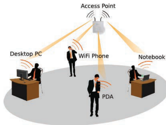
Figure 2.1: Example of a set of devices in the range of an access point (WLAN)
