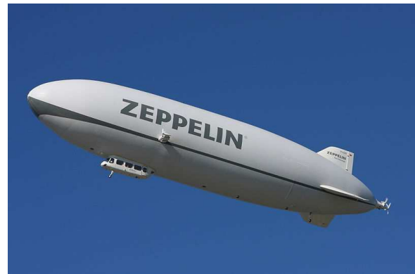
Figure 1.5: A Zeppelin NT airship. The German company recovered the construction of the Zeppelin series airship in 1990s. Different from the original rigid zeppelin airships, the modern zeppelin airships are semi-rigid. These airship can take 2 crews and 12 passengers with maximum speed 125 km/h, which is smaller than the old zeppelin.
