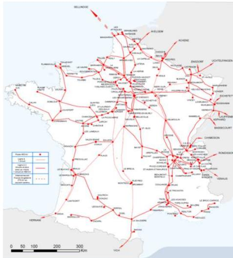
Figure 5:5 The 400kV French power transmission network (FPTN400) (RTE, 2011).
