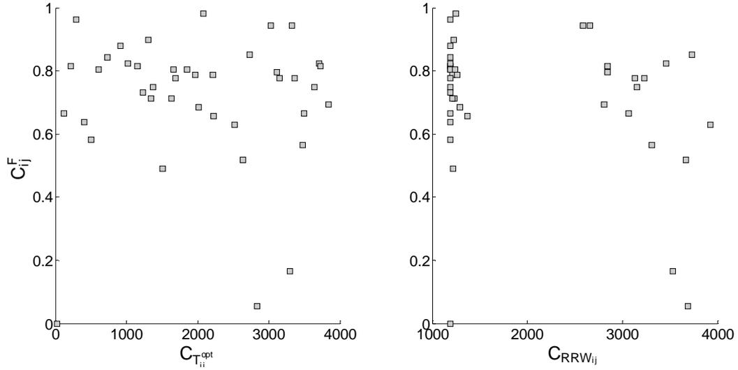
Fig. 11. Scatterplot of the Copeland scores of the optimal repair time  $C_{T_{ij}^{opt}}$  (left panel) and resilience reduction worth  $C_{RRW_{ij}}$  (right panel) with flow betweenness  $C_{ij}^F$  for the links of the IEEE 30 Bus network.
