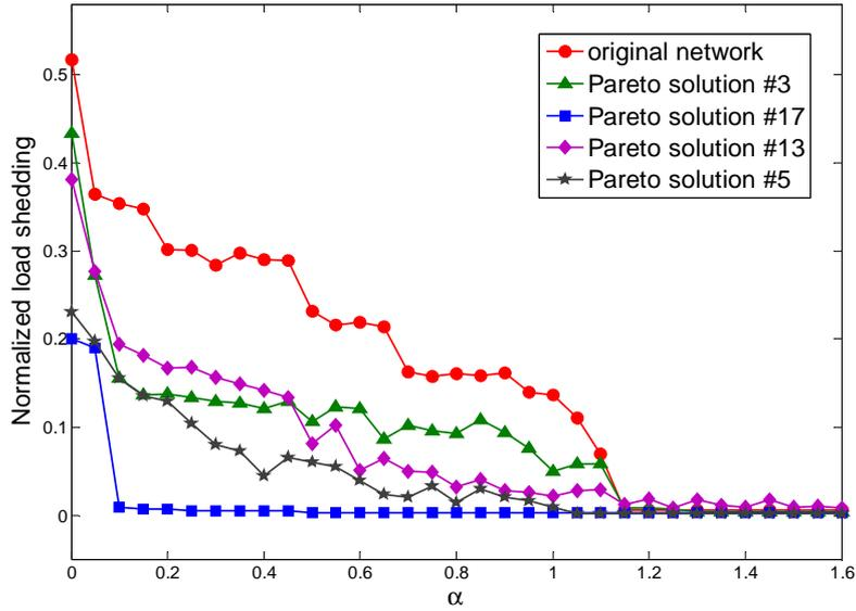
**Fig. 7.** Cascading vulnerability (normalized load shedding) evaluated by the OPA model for the five chosen networks over a range of network tolerance values  $\alpha$  under targeted initial failure.
