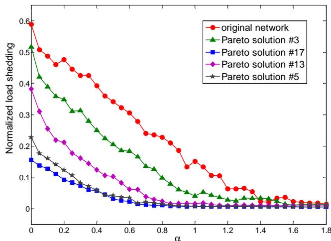
Figure 5:9 Cascading vulnerability (normalized load shedding) evaluated by the OPA model for the five chosen networks over a range of network tolerance values  $\alpha$  under random initial failure. The results have been averaged over 30 different samples.
