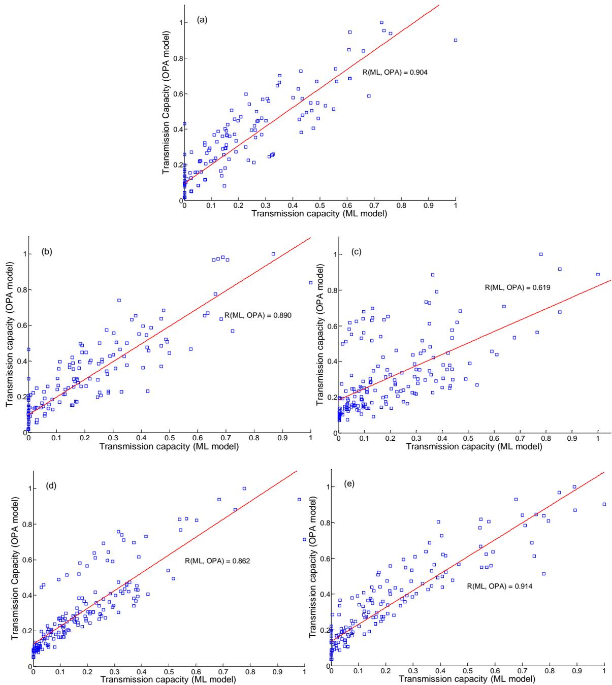
**Fig. 6.** Scatterplot of normalized node transmission capacity in ML versus OPA model using, (a) the original FPTN400; (b) Pareto solution #3 network; (c) Pareto solution #17 network; (d) Pareto solution #5; (e) Pareto solution #13. Node transmission capacity in OPA is highly correlated with transmission capacity in ML, the correlation coefficient are 0.904, 0.890, 0.619, 0.862 and 0.914 for the five networks, respectively. The solid lines represent the best fits.
