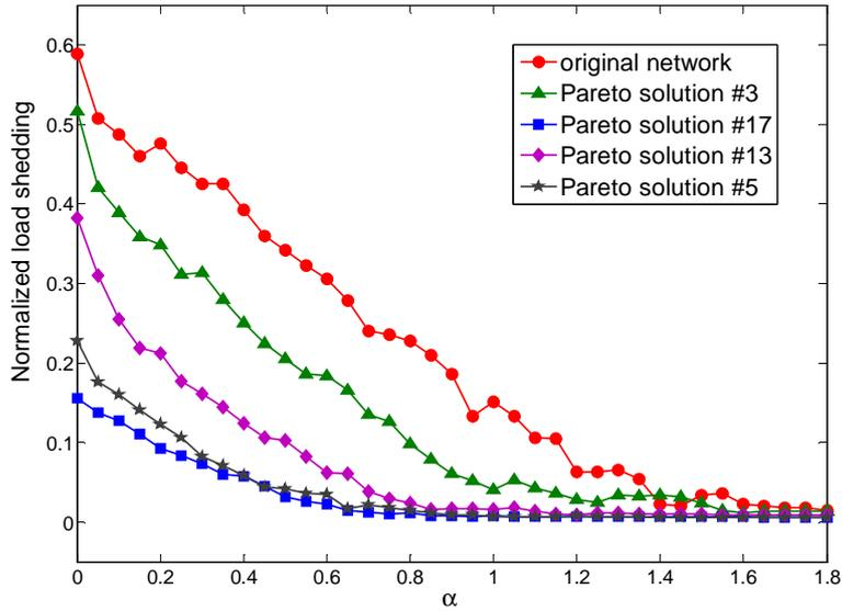
**Fig. 8.** Cascading vulnerability (normalized load shedding) evaluated by the OPA model for the five chosen networks over a range of network tolerance values  $\alpha$  under random initial failure. The results have been averaged over 30 different samples.
