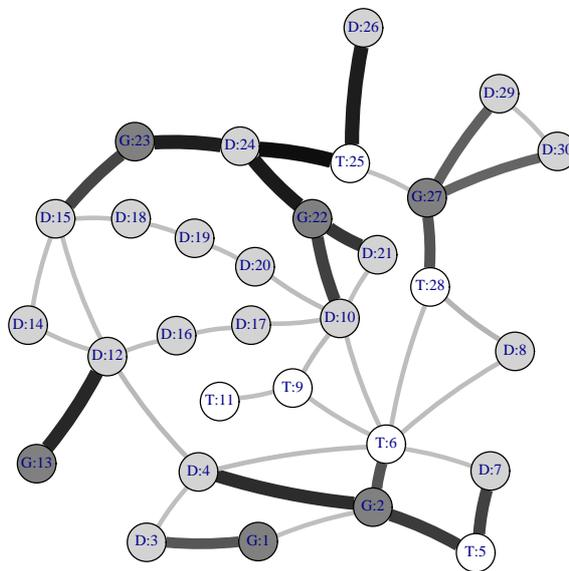
Fig. 9. Graphical illustration of the Copeland scores of the resilience reduction worth  $RRW_{ij}(\Delta t_0 = 3)$  for all IEEE 30 Bus network links. Links with higher values of Copeland score are represented as thicker and darker edges.
