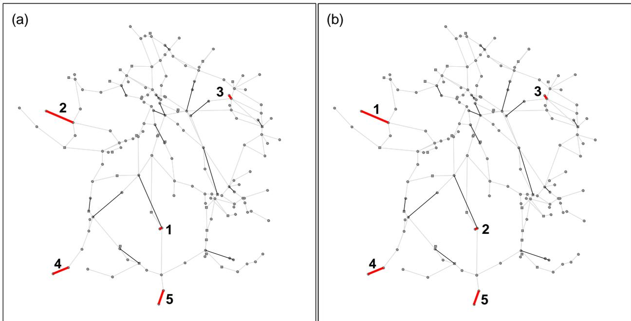
Fig. 5. Visualization of the optimal recovery plans obtained by the dispatching rule (a) and MIP solver (b) for the specific disruption scenario (10% links damaged) on the FPTN400. The numbers indicate the optimal recovery timeslots of the five arcs marked by bold solid lines; black lines correspond to other failed arcs.
