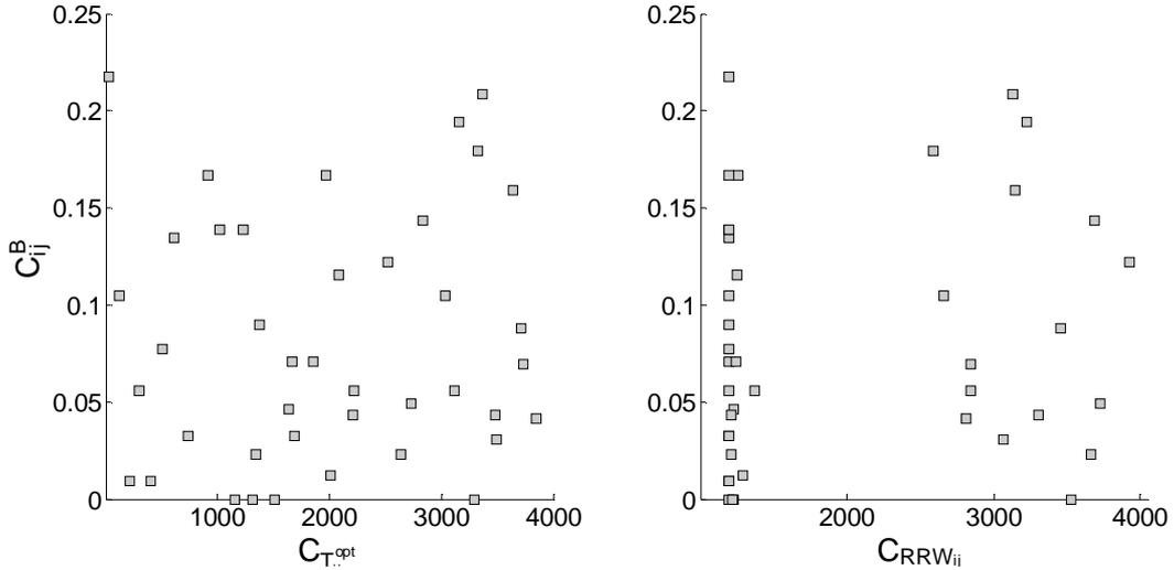
Fig. 10. Scatterplot of the Copeland scores of the optimal repair time  $C_{T_{ij}^{opt}}$  (left panel) and resilience reduction worth  $C_{RRW_{ij}}$  (right panel) with the shortest path betweenness  $C_{ij}^B$  for the links of the IEEE 30 Bus network.
