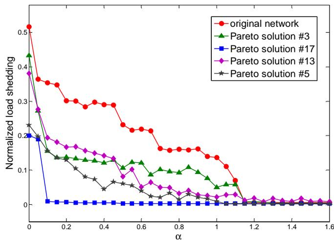
Figure 5:8 Cascading vulnerability (normalized load shedding) evaluated by the OPA model for the five chosen networks over a range of network tolerance values  $\alpha$  under targeted initial failure.
