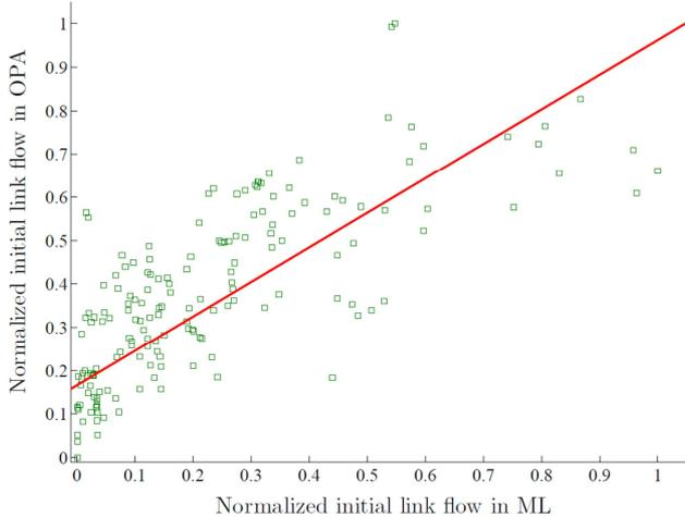
Fig. 2. Scatter-plot of the normalized initial link flows in the ML and OPA models, with reference to the 400kV French power transmission network. The initial link flow in ML is highly correlated to that in OPA ( $r_{ML,OPA}=0.77$ ). The best fit line is also shown.
