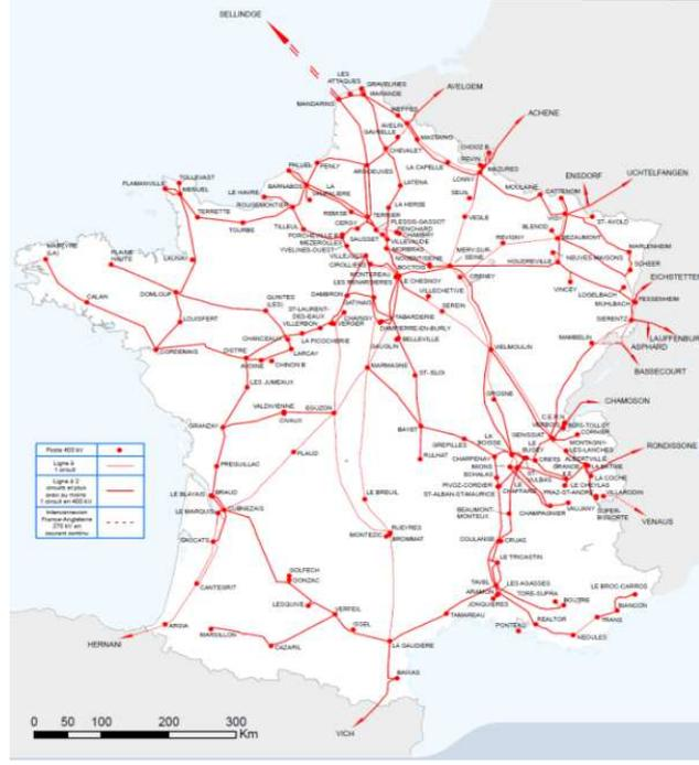
**Fig. 1.** The 400kV French power transmission network (FPTN400) <sup>(37)</sup>
