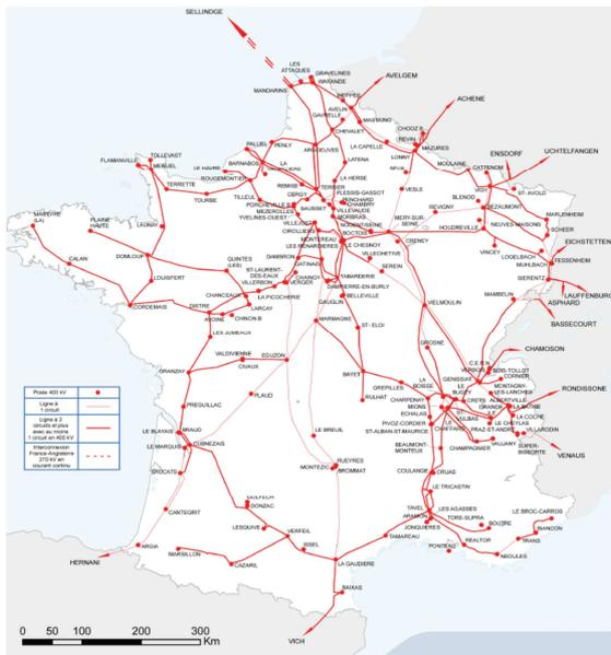
Fig. 1. The 400kV French power transmission network (FPTN400) [37].
