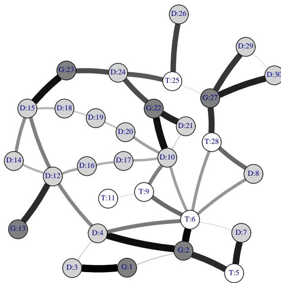
Fig. 7. Graphical illustration of the Copeland scores of the optimal repair time  $T_{ij}^{opt}$  for all IEEE 30 Bus network links. Links with higher value of Copeland score are represented as thicker and darker edges.
