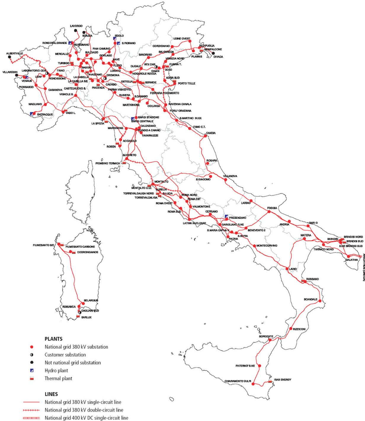
Fig. 1. The 380 kV Italian power transmission network.
