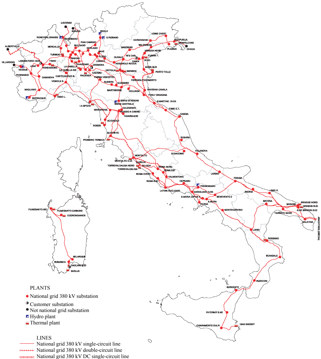
Figure 1. The 380 kV Italian power transmission network.
