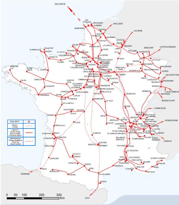
Fig. 3. The 400kV French Power Transmission Network (FPTN400) [46]
