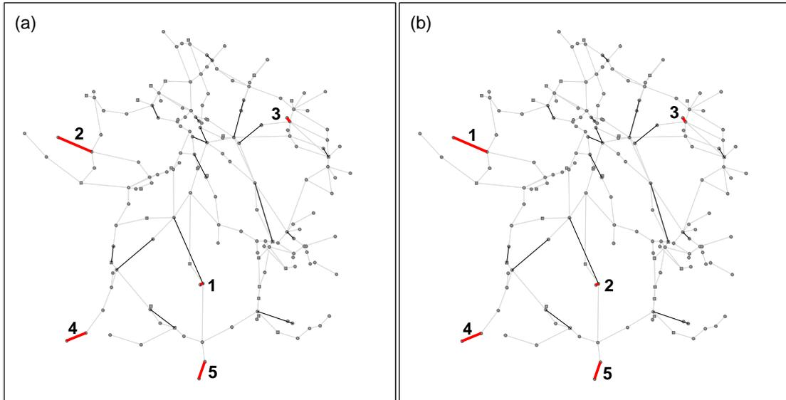
Figure 5:14 Visualization of the optimal recovery plans obtained by the dispatching rule (a) and MIP solver (b) for the specific disruption scenario (10% links damaged) on the FPTN400. The numbers indicate the optimal recovery timeslots of the five arcs marked by bold solid lines; black lines correspond to other failed arcs.
