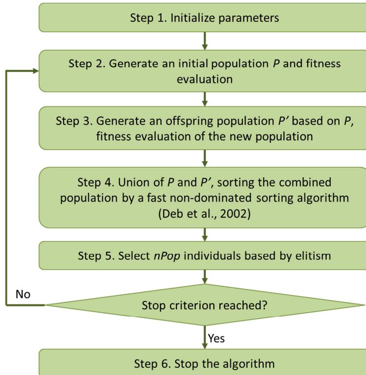
Figure 3:1 Flowchart of the common procedure of NSBDE and NSGA-II.
