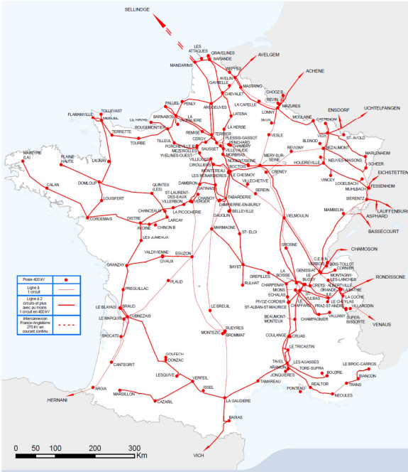
Fig. 3. The 400kV French Power Transmission Network (FPTN400) [46]
