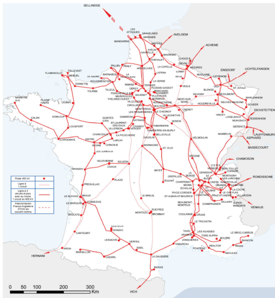
Fig. 1. The 400kV French power transmission network (FPTN400) [37].
