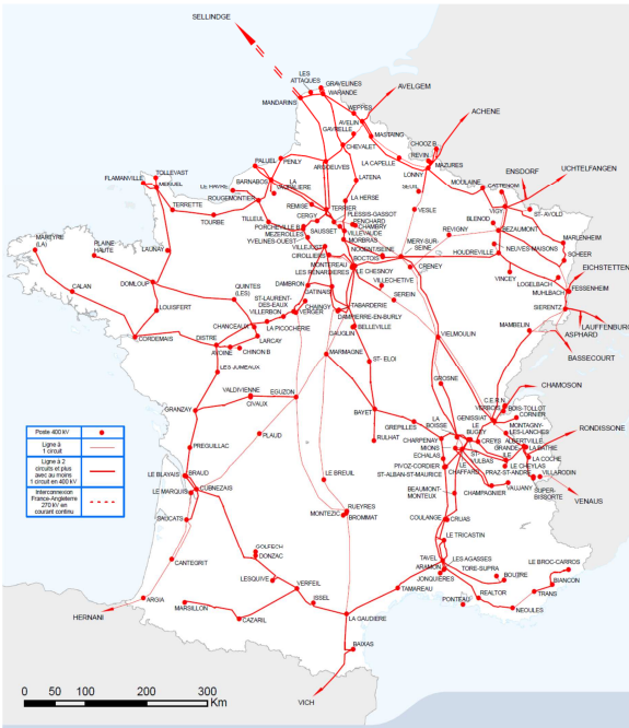
Fig. 3. The 400kV French Power Transmission Network (FPTN400) [46]
