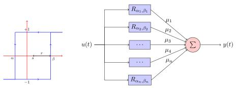
(a) Elementary Unit, a hysteron.  $\alpha$  and  $\beta$  are the thresholds for switching.
