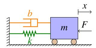
Figure 5.10: Example of a mechanical passive system.
