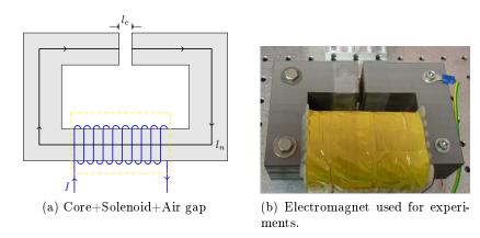
Figure 5.2: Electromagnet used to generate magnetic field.
