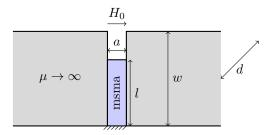
Figure 3.12: MSMA in Air Gap
