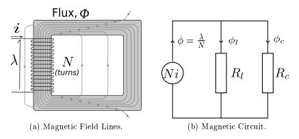
Figure B.2: Magnetic Circuit.
