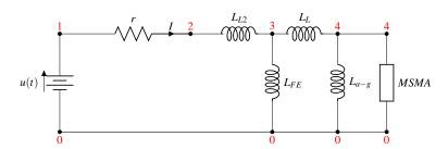
Figure 2.6: MSMA electrical subsystem
