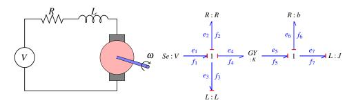
Figure 4.12: DC Motor and its Bond Graph.
