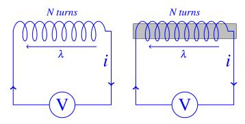
Figure B.1: Solenoid with and without material
