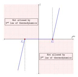
Figure 4.23: Constitutive Equation for Damper (R-element).
