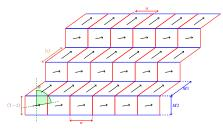
(d) If specimen is blocked, no twinning motion occurs.  $\theta$  rotates on increasing magnetic field.
