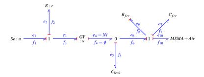
Figure 4.16: Bond graph model of reluctance circuit
