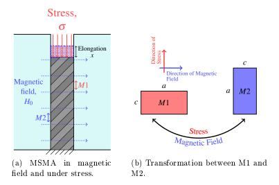
Figure 2.2: Actuation Mechanism.
