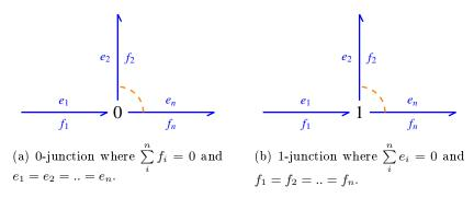
Figure 4.2: 0-junction and 1-junction. In both cases,  $\sum_{i=0}^{n} e_i f_i = 0$ .
