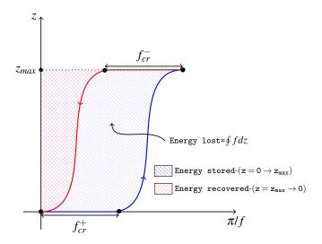
Figure 4.21: A typical hysteresis curve for MSMA.
