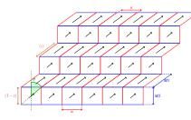
(c) After critical value of magnetic field has reached. Twinning start M1 grows at expense of M2. Domain walls  $1-\alpha$  have disappeared.
