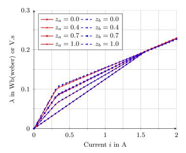
Figure 3.14: Comparaison of constitutive equations taking into account change in length of air-gap, w, as well as change in length of MSMA, l. Dashed lines show the constitutive equations when the changes in length are taken into consideration while Solid lines show the equations when the changes are assumed negligible.
