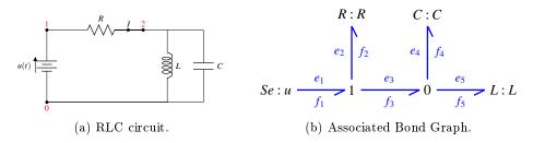
Figure 4.3: Bond Graph of RLC circuit.
