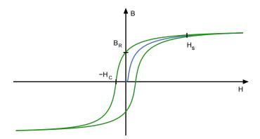
Figure 1.9: Typical hyster B-H curve which occurs in ferromagnetic materials.
