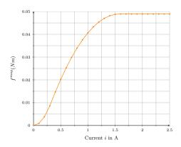
Figure 3.16: Driving force  $f^{mag}$  derived from co-energy,  $W^*_{mag}$ .
