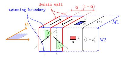
Figure 3.4: Representative volume. The direction of the magnetization vector in  $\alpha$  is in the same direction as  $H_0$ .
