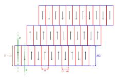
(g) On applying a very high stress with no magnetic field, only M2 is present. All M1 dissappears.
