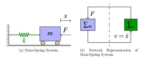
Figure 1.6: Mass-Spring and its network structure.
