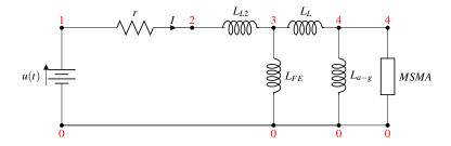
Figure 2.4: MSMA electrical subsystem
