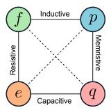
Figure 4.1: The four-element quadrangle
