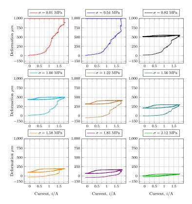
Figure 5.6: Hysteresis of actuator between current and position.
