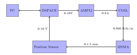
Figure 5.1: Block diagram of the experimental test bench.
