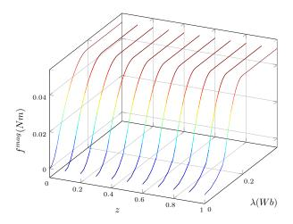
Figure 3.17: Driving force  $f^{mag}$  derived from energy,  $W_{mag}$ .
