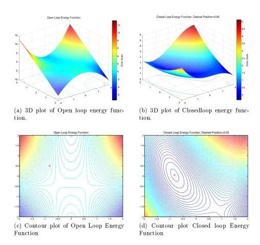
Figure 5.12: Open Loop and Closed loop of  $H_d$ . Desired Position=0.05
