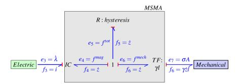
Figure 4.18: The Bond Graph of the MSMA. The "IC" field and the transformer "TF" act as energy converting ports.
