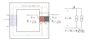
(b) Equivalent Parallel Circuit.
