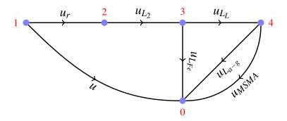
Figure 2.7: Linear graph of MSMA actuator
