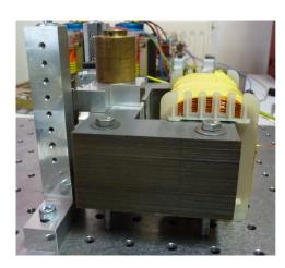
Figure 5.4: Assembled electric circuit and mechanical structure to make a crude actuator.
