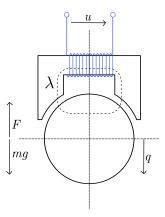
Figure 5.11: Magnetic Levitation System
