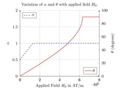
Figure 3.6: Variation of  $\alpha$ ,  $\theta$  with applied  $H_0$
