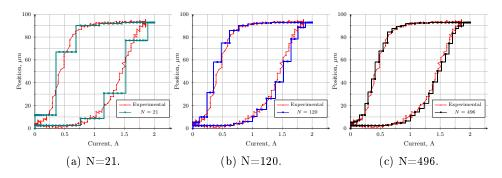
Figure 5.7: Preisach Model with different number of hysterons to model experimental curve. N is the number of hysterons.
