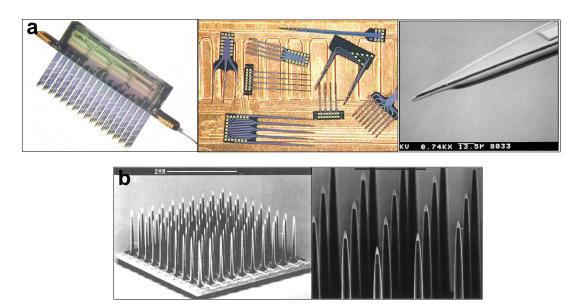
**Figure 1.12:** a) the Michigan electrodes: 64-site probes assembled in 3D structures, a variety of silicon probes on the back of a U.S. penny and SEM image of the recording site (from [43]). b) The Utah array and the insulation coated electrodes with exposed platinum tips (from [48]).
