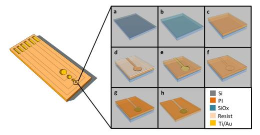
Figure 2.5: Schematic illustration of the main steps for the fabrication of polyimide-based electrodes.
