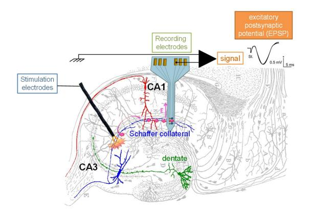
**Figure 4.6:** Cross section of the hippocampus (with its main regions of interest) and the placement of the stimulation and recording electrodes with the configuration used in the reported experiments (adapted from [12]).
