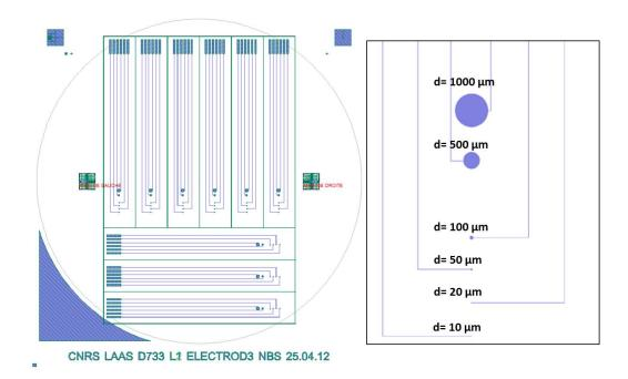
Figure 2.2: Mask design for the prototype polyimide-based electrodes and electrode sizes.
