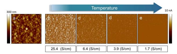
Figure 3.28: a) Contact mode AFM topography of PEDOT layer formed under PD mode (scan of potential from -0.9 V to 1.2 V, scan rate 0.025 V/s, 10 cycles) and current corresponding images with C-AFM under an applied potential of 50 mV at the temperature of b) 25, c) 50, d) 100, e) 150°C recorded after  $\frac{1}{2}$ h, over a scanned area of 10  $\mu$ m x 10  $\mu$ m. Under every image the corresponding calculated conductivity is given.
