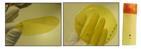
Figure 2.4: Peeled off polyimide-based electrodes used for preliminary tests.
