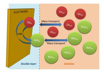
**Figure 10:** Schematic image of the mass transport and charge transfer at the electrode/solution interface.
