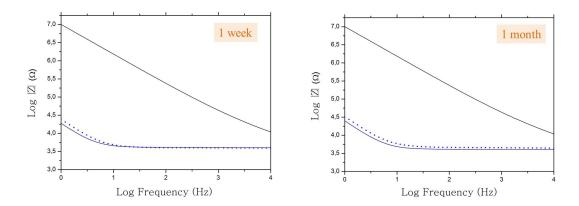
Figure 3.30: Impedance curve before (black) and after (blue) PEDOT:PSS polymerization and after ageing (dotted blue), over a frequency range of  $10^{0}$ - $10^{4}$ Hz, after 1 week and 1 month of ageing process at  $70^{\circ}$ C (f = 9,8).
