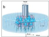
**Figure 1.11:** a) SEM Micrographs of microelectrodes wires with an insulation layer consisting of Parylene-C and microelectrode tip regions (from [40]). b) The microwire tetrode (from [41]).
