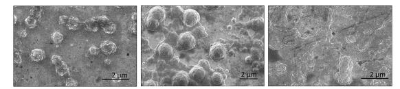
**Figure 3.10:** Formation of PEDOT nuclei, overlapping and full covering of the surface during the polymerization progress.
