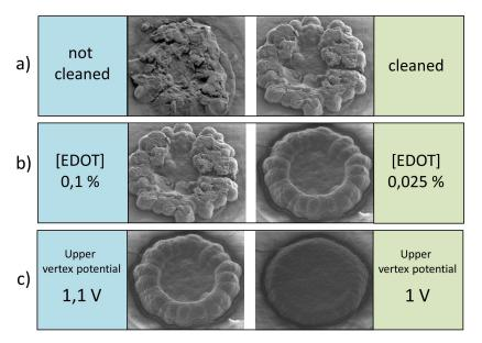
Figure 3.17: SEM images of different morphologies of PEDOT:PSS layers related to different electrochemical deposition parameters.
