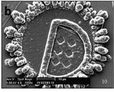
Figure 3.6: Electrochemical PE-DOT deposition through a) galvanostatic and b) potentiostatic conditions[13].
