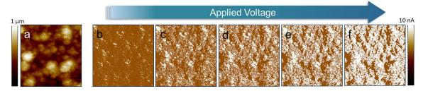
Figure 3.32: a) Contact mode AFM topography of PEDOT:PSS layer formed under PD conditions (scan of potential from -0.7 V to 1.15 V, scan rate: 0.05 V/s, 10 cycles) and current corresponding images with C-AFM at b) 10 mV, c) 50 mV, d) 100 mV, e) 200 mV, f) 500 mV, after 1 month at  $70^{\circ}C$ , recorded over a scanned area of 10  $\mu$ m x 10  $\mu$ m.
