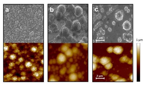
**Figure 3.14:** SEM and AFM images of the PEDOT:PSS films formed under (a) PD, (b) PS and (c) GS conditions.
