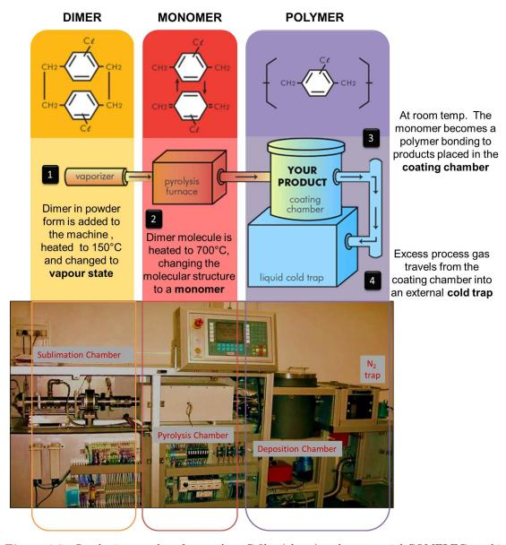
**Figure 2.7:** Synthesis procedure for parylene-C film (above) and commercial COMELEC machine for the CVD deposition of parylene and its main parts (below).
