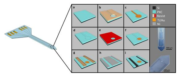
Figure 2.12: Schematic illustration of the main steps for the fabrication of the parylene-based microelectrodes.
