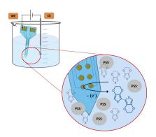
Figure 3.9: Schematic illustration of the first steps of the electrochmical polymerization process.
