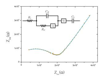
Figure 3.24: Nyquist diagram for a PEDOT-modified 10  $\mu$ m diameter electrode and related fitting curve using the equivalent circuit.
