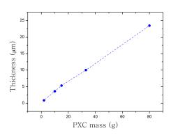
Figure 2.10: Relation between the starting mass of PXC precursor and the thickness of the obtained film.
