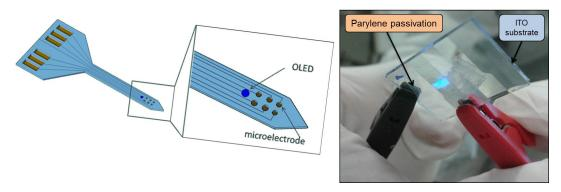
Figure 5.2: Schematic representation of the OLED integrated electrode and first test of blue (470 nm) OLED encapsulation into parylene-C.
