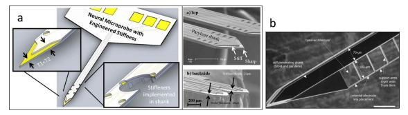
Figure 1.23: a) parylene-based sharp-tipped microprobes, with shanks of 2 mm-long, 20  $\mu$ m-thick and 380  $\mu$ m-wide[132]. b) parylene-based open-architecture with a thick shank and an integrated thin lateral platform [129].
