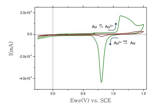
Figure 3.11: Au electrode voltammogram before (red) and after (green) electrode area cleaning by cyclic voltammetry with a potential scan from -0.25 V to 1.5 V, at the scan rate of 0.5 V/s, in  $\rm H_2SO_4$  [0.5 M] solution.
