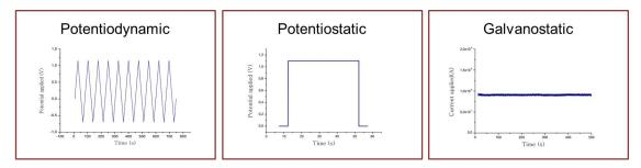
Figure 3.3: The three electropolymerization routes.
