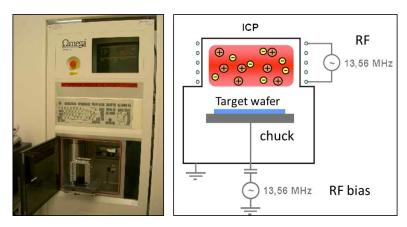
Figure 8: The machine Aviza Technology Omega 201 used in our process (on the left) and a scheme of the machine functioning (on the right).
