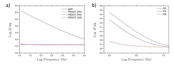
**Figure 3.22:** EIS over a range of a)  $10^1$ - $10^4$  Hz and b) 1- $10^1$  Hz, for a 100  $\mu$ m-diameter electrode in a NaCl 0.9% solution for different electropolymerization routes.
