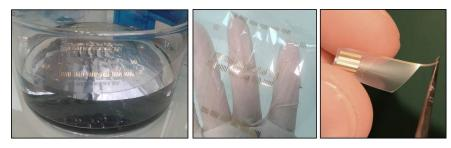
Figure 2.13: Release of PXC-based devices in water and final appearance of the electrode.
