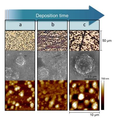
**Figure 3.15:** Optical Microscope, SEM and tapping mode AFM images of the PEDOT:PSS films formed under PS mode at 0.90 V for (a) 5 s, (b) 10 s, (c) 50 s (the scales are the same for the three images).
