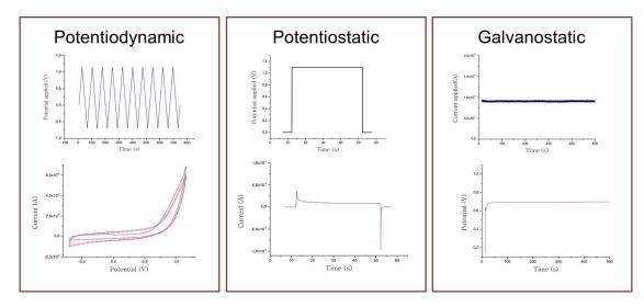
**Figure 3.7:** Representation of the three routes of polymerization with the corresponding current (or potential) curves.
