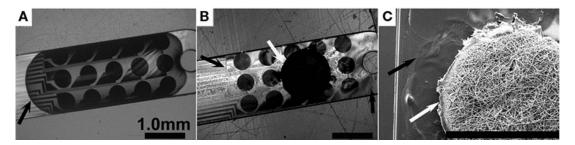
Figure 1.14: A) Optical micrographs of the tip of a microeletrode array coated with PEGPCL hydrogel and B) coated with PEGPCL hydrogel-EFM composite. C) SEM micrograph of the tip of an MEA coated with PEGPCL hydrogel-PCL EFM composite (from [75]).
