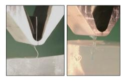
Figure 2.18: Insertion test in Agarose gel before (left) and after (right) the silk deposition.
