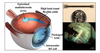
Figure 1.22: Placement and components of envisioned intraocular retinal prosthesis and parylene MEAs tacked to the right retina[63].
