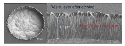
Figure 2.15: Etching parylene residues on the sidewalls before stripping the resist.
