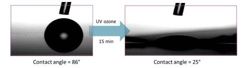
Figure 2.11: Contact angle of water on PXC before and after the UV ozone treatment.
