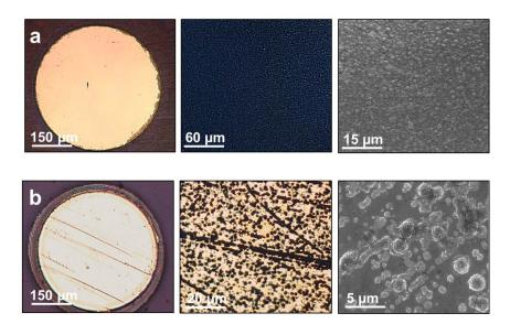
Figure 3.13: Optical Microscope and SEM images of the PEDOT:PSS films formed on a) very smooth and b) scratched gold surface.
