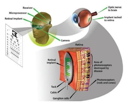
Figure 1.31: Schematic illustration of the artificial retina functioning.
