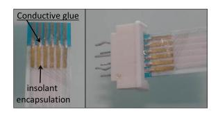
**Figure 2.9:** Electrical connection for the parylene electrode.
