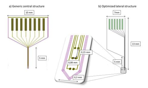
**Figure 2.8:** The two main configurations of parylene-based devices: a) central octatrode and b) lateral hexatrode (optimized for the *in vivo* recording set-up).
