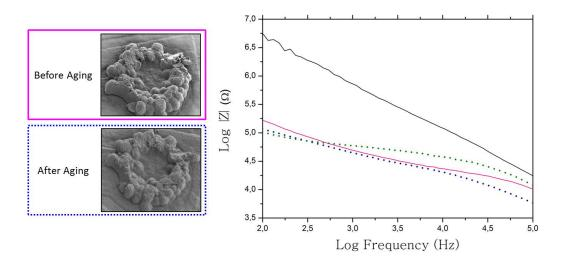
Figure 3.31: Impedance curve before (black) and after (pink) PEDOT:PSS deposition, suddenly after the ageing process (dotted blue), and left 1 day at room temperature after the ageing process (dotted green) over a frequency range of  $10^2$ - $10^5$ Hz.
