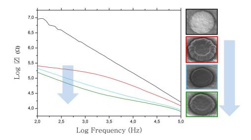
Figure 3.23: Impedance lowering (over a range of  $10^2$ - $10^5$  Hz) and related morphology for different deposition conditions presented in Section 3.4.5 for 10  $\mu$ m-diameter electrodes.
