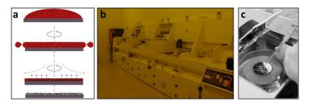
Figure 3: a) spin coating scheme, b) and c) spin coaters available in our laboratory.
