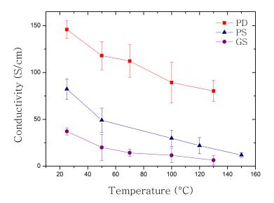
Figure 3.29: Variation of conductivity with temperature for three PEDOT:PSS layers electrode-posited under PD (red), PS (blue) and GS (violet) conditions.
