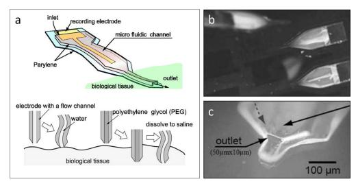
**Figure 1.25:** a) Takeuchi *et al.*[64] parylene-based neural probe with microchannel; b) filling of the channel with PEG to increase the stiffness; c) the limited PEG exposed area to the physiologic liquid through the outlet should reduce the dissolution time.
