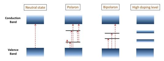
Figure 3.18: Energy level diagram of conductive polymers. Dashed red arrows indicate possible electronic transitions caused by light absorption.
