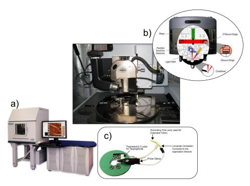
Figure 16: The used equipment: a) the cage, vibration isolation platform and the electronic control with computer; b) the AFM "head" and a scheme of its composition; c) the tip holder for the conductive module.
