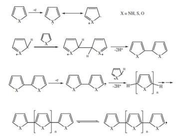
Figure 3.4: Mechanism for heterocycle polymerization via electrochemical synthesis[7].
