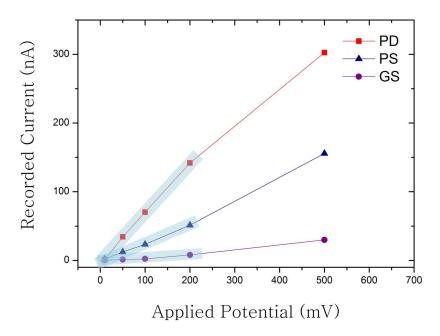
Figure 3.27: C-AFM I-V curve for the samples electropolymerized by three different ways, recorded over a scanned area of 10  $\mu$ m x 10  $\mu$ m. The ohmic zone is underlined in light blue.
