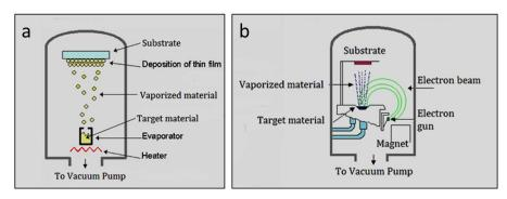
Figure 7: Scheme of the PVD machine in the case of a) resistance heating evaporation and b) electron beam evaporation.
