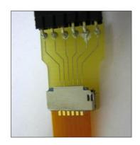
Figure 2.3: Connection for the polyimide prototype electrode.
