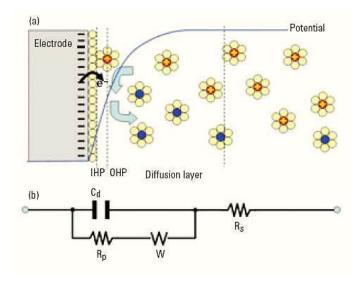
Figure 12: Schematic image of the a) interface electrode/solution and b) associated Randless circuit.
