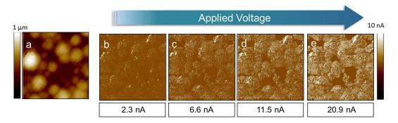
**Figure 3.26:** Contact mode AFM topography (a) of PEDOT:PSS layer formed under PS conditions (0.9 V for 50 s) and current corresponding images with C-AFM at (b) 10 mV, (c) 50 mV, (d) 100 mV, (e) 200 mV, recorded over a scanned area of 10  $\mu$ m x 10  $\mu$ m.
