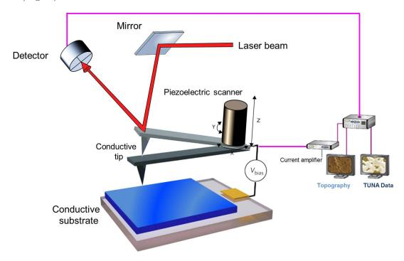
Figure 15: Schematic drawing of a conductive AFM (adapted from [4, 5, 6]).
