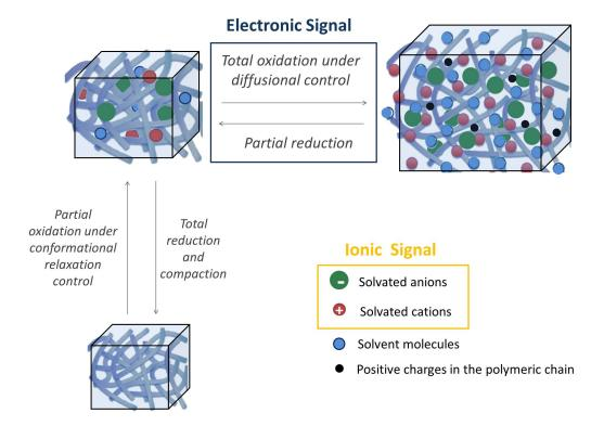
Figure 3.2: Schematic representation of the reversible variation of volume associated with the electrochemical-switching conducting polymers. Changes in free volume are mainly due to two effects: electrostatic repulsions between fixed positive charges and exchange of cations, anions, and solvent molecules between the polymer and the solution.
