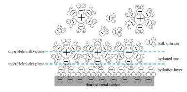
Figure 1.15: The electrode-electrolyte interface [47].
