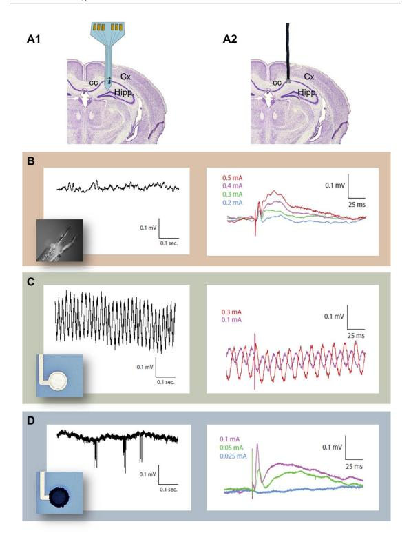
Figure 4.9: Scheme of the placement of A1) parylene-based hexatrode with 3 pristine microelectrodes and 3 PEDOT-modified microelectrodes and A2) twisted NiCr electrode, across the pyramidal layer of area CA1. Signal recording and magnification of LFPs at different stimulation intensities using B) the NiCr twisted electrode, C) pristine Au parylene-based microelectrode, D) PEDOT:PSS modified parylene-based microelectrode. Cx: Cortex, cc: corpus collosum, Hipp.: hippocampus.
