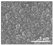
Figure 3.16: SEM images of a PEDOT:PSS layers on a 10  $\mu$ m-diameter electrode (left) and 50  $\mu$ m-diameter electrode (right).
