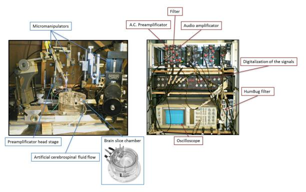
**Figure 4.1:** Picture of the experimental set-up for recording signals in brain slices, depicting the slice chamber and all the components for the signal digitalization.
