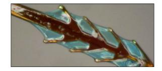
Figure 1.26: Silk coated probe with tip shown. Silk solution was mixed with blue dye prior to coating for better visualization[138].
