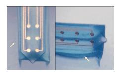
Figure 2.17: Optical microscope image of silk deposition on the backside of the probe.
