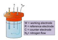
Figure 9: Scheme of a classical three-electrode cell.
