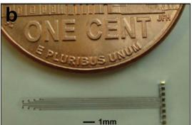
Figure 1.13: Two examples of flexible implantable electrodes fabricated on a) polyimide (from [55]) and b) parylene (from [62]).
