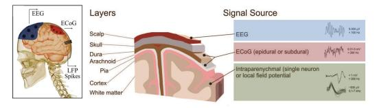
Figure 1.6: Placement of implanted and non-implanted recording devices at different depths, over, onto or inside the brain and the related recorded signals (adapted from [16, 17]).
