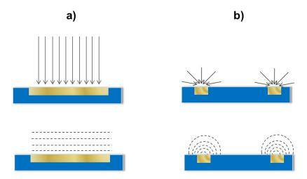
Figure 11: Diffusion flux and diffusion profile for a) plane conventional electrode (linear diffusion) and b) disk microelectrode (hemispherical diffusion).
