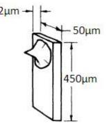
Figure 17: Cantilever dimensions.
