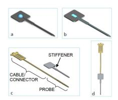
Figure 1.24: Process to assemble a flexible polymer probe to a silicon stiffener with polyethylene glycol[134].
