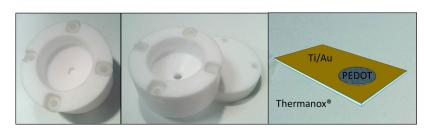
**Figure 2.26:** Electrochemical Teflon® cell and resulting Thermanox® coverslip after the PE-DOT:PSS polymerization over a 3 mm-diameter area.
