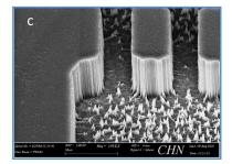
Figure 2.16: Cutting of electrode edges by plasma etching (a) before and (b) after chemical etching of the Nickel mask; (c) example of similar residues in the literature[27].
