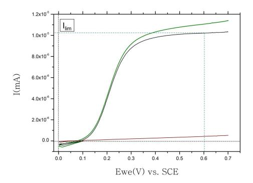
Figure 3.12: LSV from 0 V to 0.7 V, in  $K_4Fe(CN)_6$  [10 mM] and KCl [0.1 M] in PBS (green curve), in KCl [0.1 M] in PBS (red curve) and subtraction curve (black curve).
