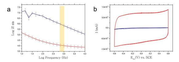
**Figure 3.21:** a) Electrochemical mean impedance spectroscopy over a range of  $10^1$ - $10^4$  Hz and related error bar and b) charge capacity for the pristine gold electrode (blue) and for the PEDOT-modified electrode (red) for a 10  $\mu$ m diameter electrode in a NaCl 0.9% solution.
