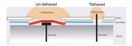
Figure 1.21: Tethered and un-tethered implantation techniques: the un-tethered set-up is ensured by adding artificial dura on top of the implant, separating the implant from the skull. In contrast, tethered implant is glued to the sealant materials (from [122]).
