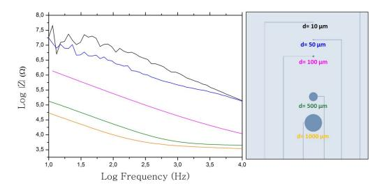
Figure 3.20: Mean impedance of gold electrode with related error bar for different electrodes diameters: 10  $\mu$ m (black), 50  $\mu$ m (blue), 100  $\mu$ m (pink), 500  $\mu$ m (green), 1000  $\mu$ m (yellow).
