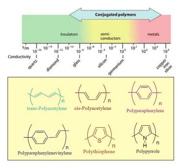
Figure 3.1: Conductivity of conductive conjugated polymers compared to metals, semiconductors and insulators (above) and some examples of conductive polymers chemical structures (below).
