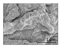
Figure 5.1: SEM image of CNTs-PEDOT:PSS embedded electrochemical deposited on a gold electrode.
