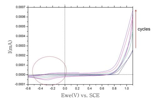
**Figure 3.8:** Cyclic voltammetry for polymerization for a 50  $\mu$ m-diameter electrode: 4 cycles from -0.7 V to 1.1 V, scan rate = 10 mV/s.
