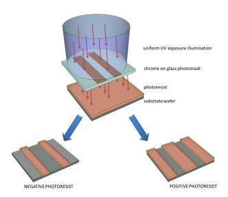
Figure 4: Scheme of the main processes in the photolithography.
