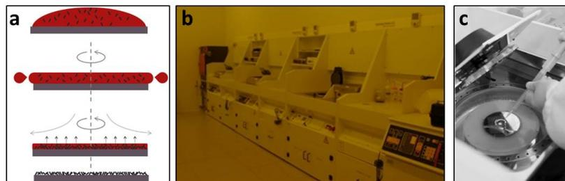
**Figure 3:** a) spin coating scheme, b) and c) spin coaters available in our laboratory.
