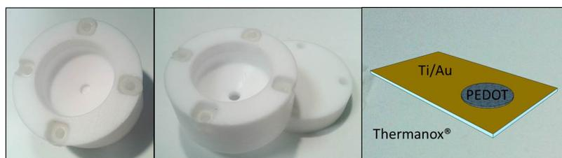
**Figure 2.26:** Electrochemical Teflon® cell and resulting Thermanox® coverslip after the PEDOT:PSS polymerization over a 3 mm-diameter area.
