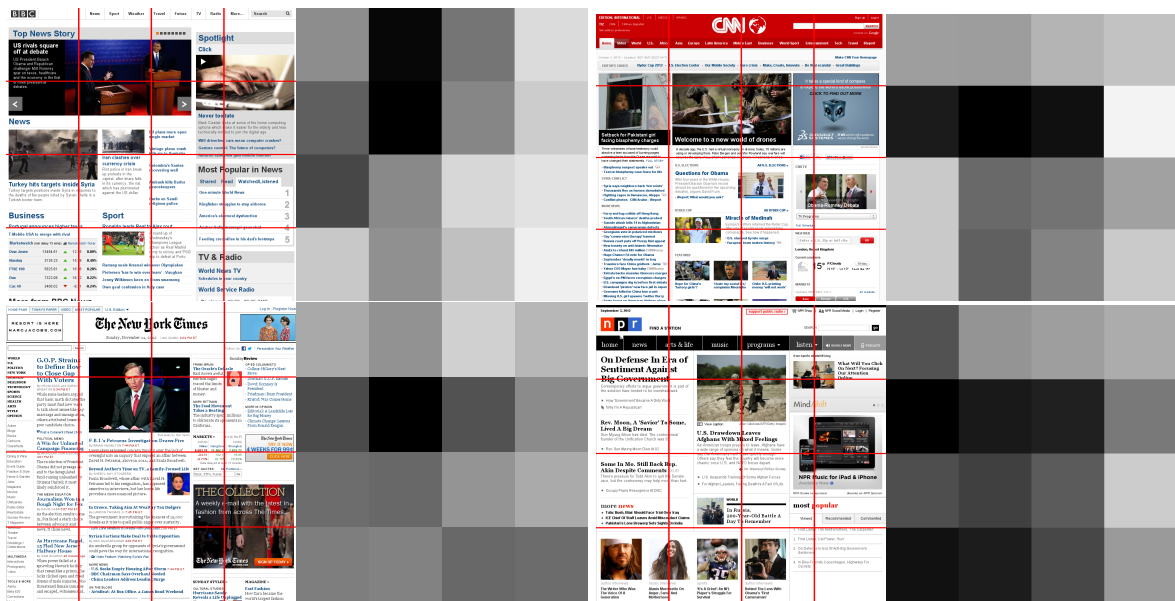
Figure 4.5: Important change maps for the homepages of BBC, CNN, New York Times and NPR. (left) Webpage screenshot with webpage regular segmentation blocks (red lines). (right) Absolute values of the eigenvector of the dominant eigenvalue of the distance non-diagonal matrix learned by our method with versions crawled during 5 days and without human supervision (higher values are darker).
