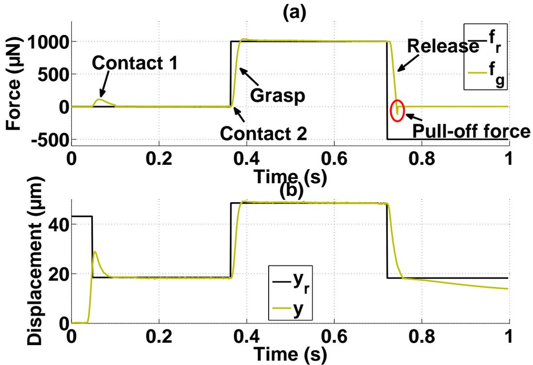
FIGURE 4.11: Experimental results for the Sliding Mode Impedance Control (SMIC) with on-line estimation of the environment parameters: (a) force response compared to the reference force, (b) position response compared to  $y_r$ .
