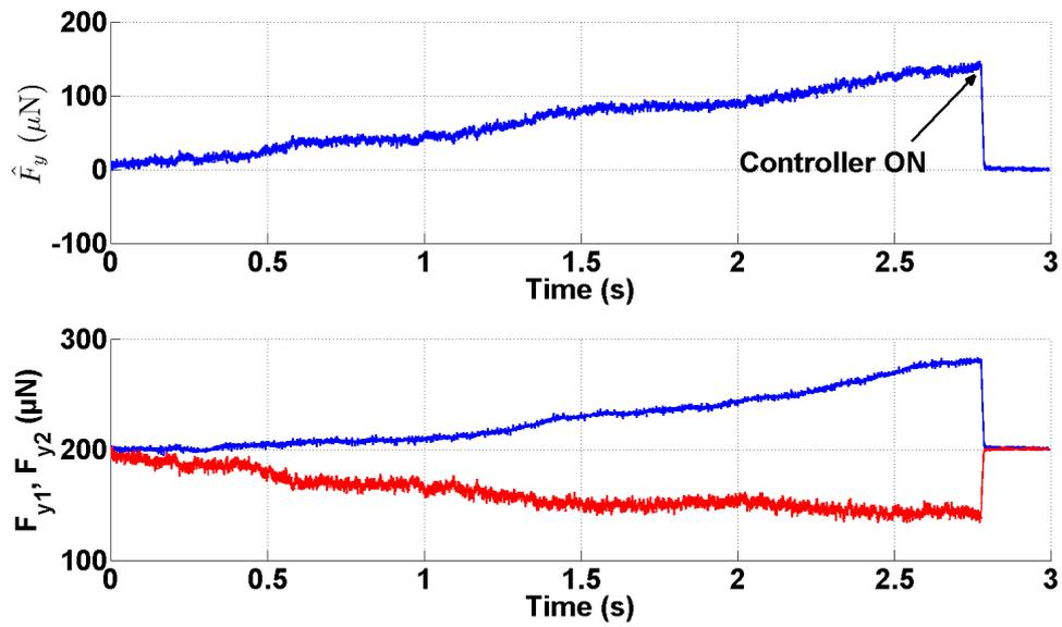
FIGURE 5.16: Experimental results for the automated guiding of a rigid micropart inside a rail showing the estimation of the contact force  $\hat{f}_y$  and the gripping forces.
