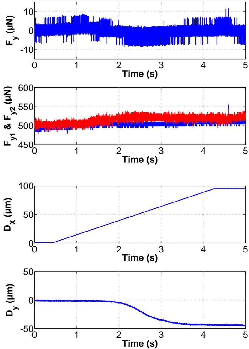
FIGURE 5.13: Experimental results for the automated guiding of a rigid micropart inside a rail showing the estimation of the lateral contact force,  $\hat{f}_y$ , and the gripping forces, the Nanocube displacement along the X axis,  $D_x$ , and the NanoCube displacement along the axis of correction Y,  $D_y$ .
