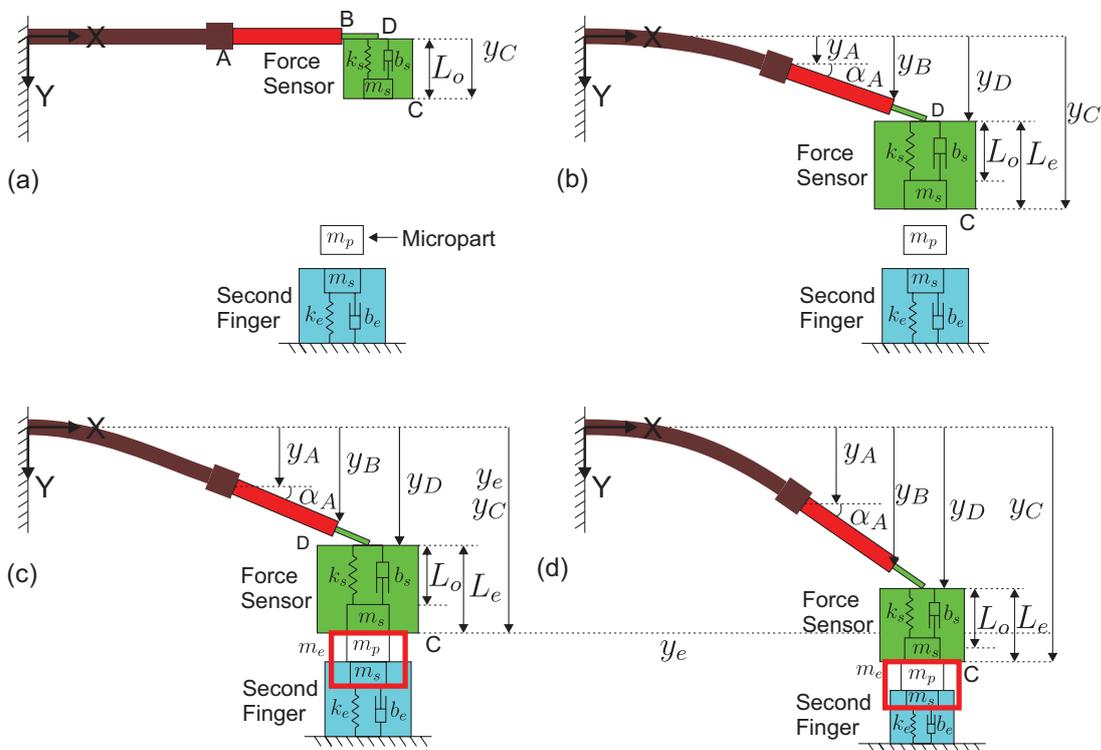
FIGURE 3.20: Equivalent dynamic scheme of the constrained motion of one of the TFSM fingers in four cases: (a) no motion without contact and without any applied voltage ( $F_s = 0$  and  $U = 0$ ) (b) free motion with an applied voltage to the finger ( $F_s = 0$  and  $U \neq 0$  the same case considered in Figure 3.18-(c)), (c) just at the transition between free motion and constrained motion ( $F_s = 0$ ) and (d) constrained motion after contact ( $F_s \neq 0$ ).
