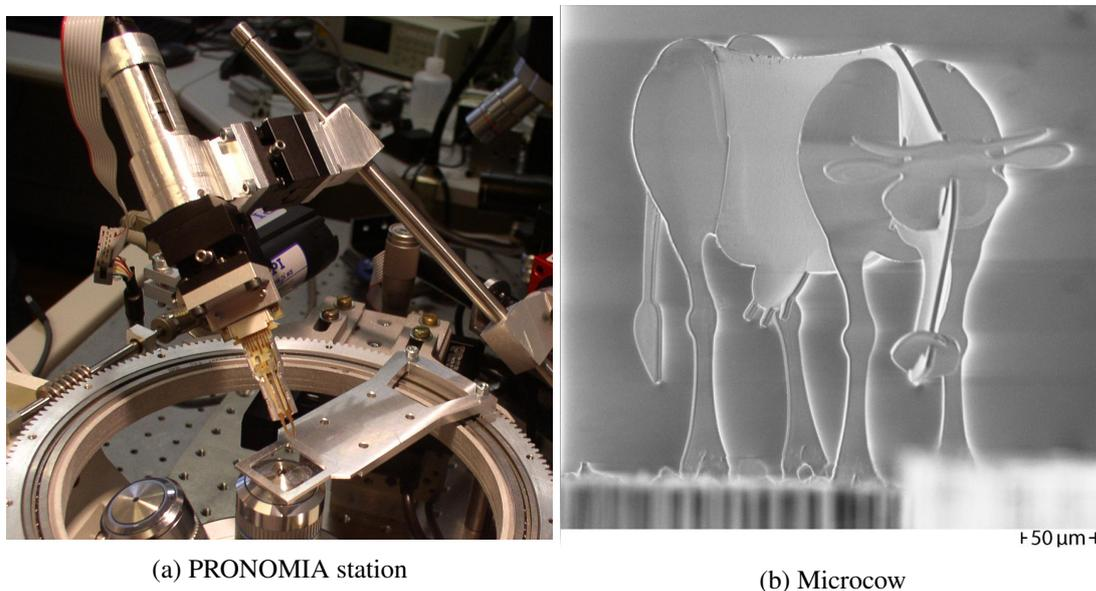
FIGURE 1.13: PRONOMIA microassembly station [62] and the assembled microcow.
