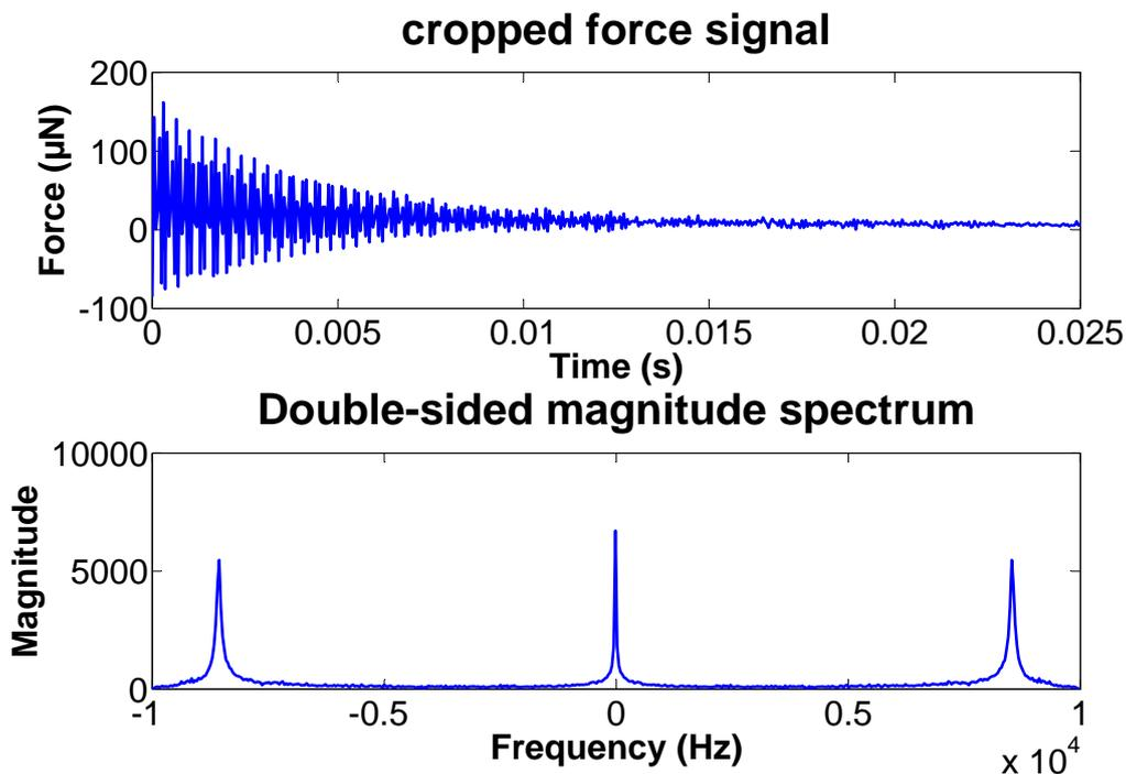
FIGURE 2.15: The time signal and the FFT signal of the signal measured by the force sensor when free vibrations are applied to the force sensor.
