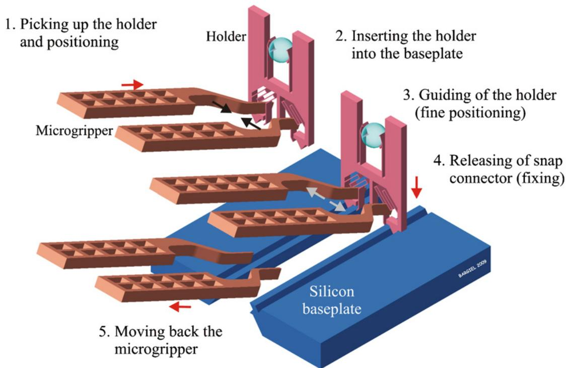
FIGURE 1.6: General concept of holder assembly based on the use of a robotic active microgripper as presented in [10]. The geometry of a gripping tool, performing the insertion and displacement of the holder within the rail of the baseplate, is illustrated.
