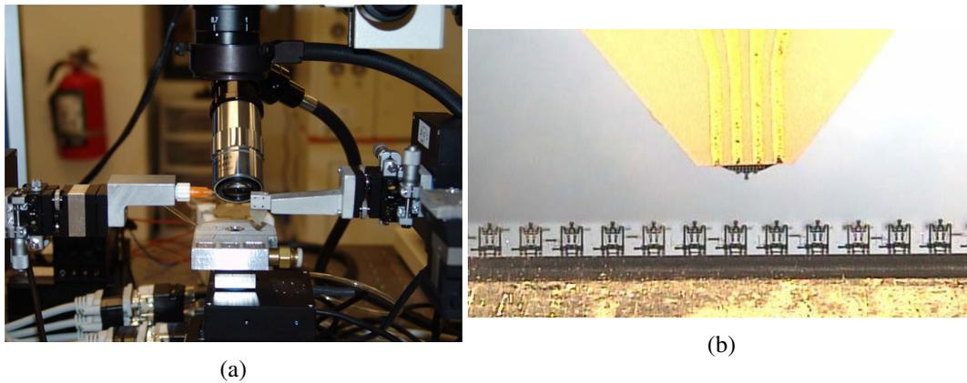
FIGURE 1.21: (a) The robotic station of the system and (b) the results of the automated open loop microassembly of 12 microparts using a passive microgripper (*jammer*) and calibrating the robotic station.
