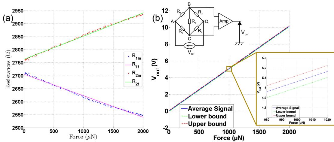
FIGURE 2.13: (a) The variation of the strain gauges resistances relative to an applied force on the tip of the force sensor.  $R_{1m}$  and  $R_{2m}$  are the measured values of resistances in experiments and  $R_{1f}$  and  $R_{2f}$  are the approximated linear variation of the resistances and (b) The variation of the readout voltage from the Wheatstone Bridge,  $V_{out}$ , for a referenced voltage of  $V_{ref} = 5\text{V}$  and amplification gain,  $A = 100$ , relative to an applied force.
