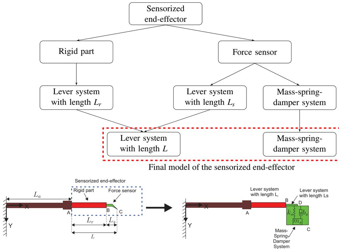
FIGURE 3.15: Equivalent scheme of the sensorized end-effector.
