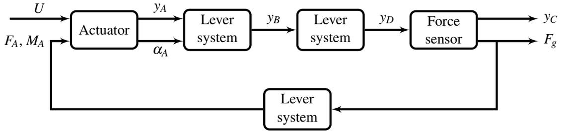
FIGURE 3.21: Bloc diagram to show the method to determine the constrained motion model of the TSFM. Notice that  $y_A$  and  $\alpha_A$  are coupled but their separation is done to clarify the parameters needed for the model.
