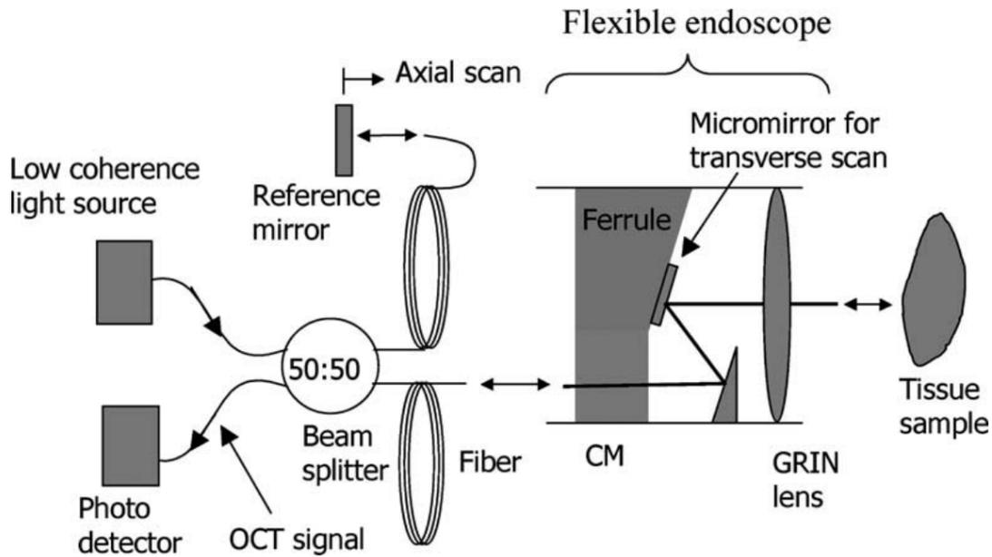
FIGURE 1.2: Schematic of the MEMS-based endoscopic OCT system. CM is the collimator. The OCT signal is the combination of the reference source and the reflected light from the sample, which creates the interference pattern. The external reference mirror moves for axial scan of the sample [185].
