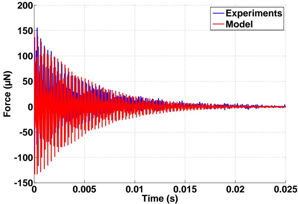
FIGURE 2.16: The time signal of the force sensor compared to the model after fitting the damping coefficient.
