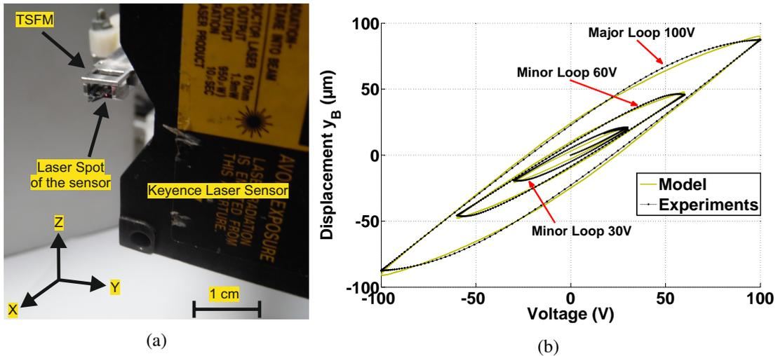
FIGURE 3.23: (a) Experimental setup used for the identification of the static parameters of the actuators; (b) Comparison between the Bouc-Wen static hysteresis model and experimental results for many sine voltages with three different amplitudes 30V, 60V and 100V at a frequency 0.1 Hz.
