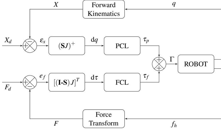
FIGURE 5.8: Hybrid force/position control diagram as defined in [53].
