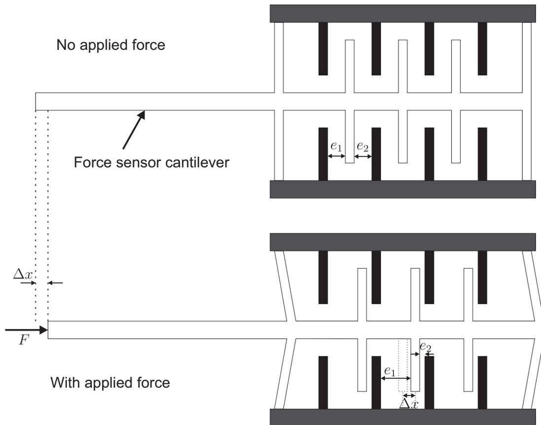
FIGURE 2.4: Differential capacitors used in electrostatic sensors.
