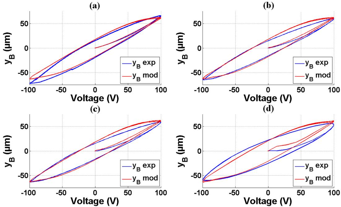
FIGURE 3.26: Comparison between the displacement model of the tip B  $y_B$  given in Equation (3.15) and experimental results for many sine voltages with an amplitude of 100V and with different frequencies where no force is applied: (a) 10Hz, (b) 50Hz, (c) 100Hz and (d) 500Hz.
