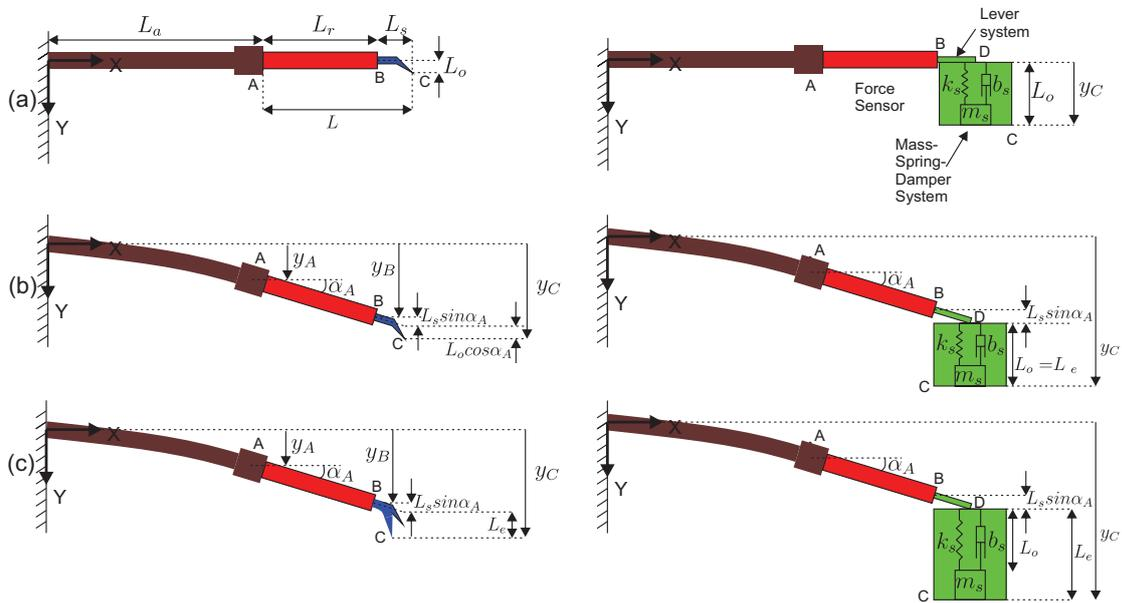
FIGURE 3.18: Equivalent scheme of the free motion of one smart finger: (a) without any applied voltage ( $U = 0$ ), (b) voltage is applied (quasi-static behavior), (c) voltage is applied (dynamic behavior). For each of the three cases, at left the scheme of the gripper and at right the scheme of gripper after replacing the force sensor by a lever system connected to a mass-spring-damper system.
