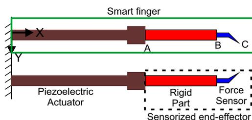
FIGURE 3.3: Complete scheme of the two-smart-fingers microgripper (TSFM).
