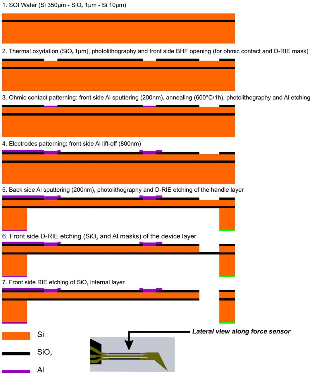
FIGURE 2.9: Microfabrication process flowchart.
