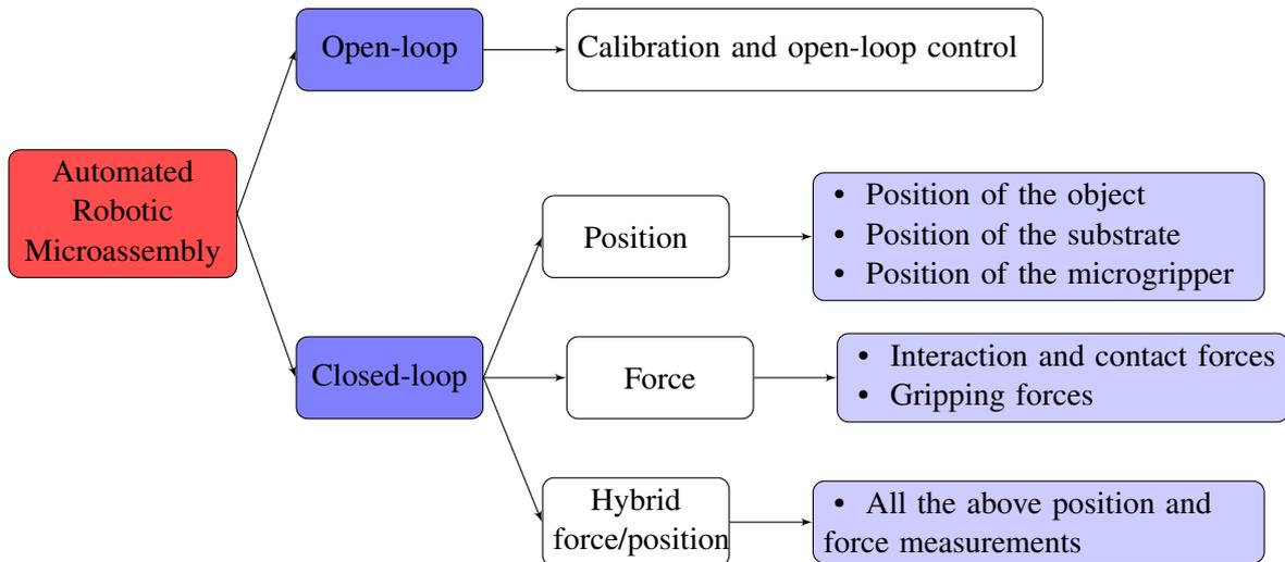
FIGURE 4.1: The different approaches for the automation of the microassembly tasks.
