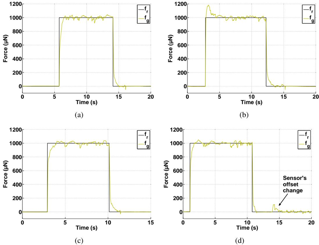
FIGURE 4.4: Experimental results of the explicit force control using PI controller for four different values of proportional and integral gains  $K_p$  and  $K_i$ : (a)  $K_p = 0.3$  and  $K_i = 0.6$ , (b)  $K_p = 0.4$  and  $K_i = 1$ , (c)  $K_p = 0.2$  and  $K_i = 0.5$ , (d)  $K_p = 0.3$  and  $K_i = 0.7$ .
