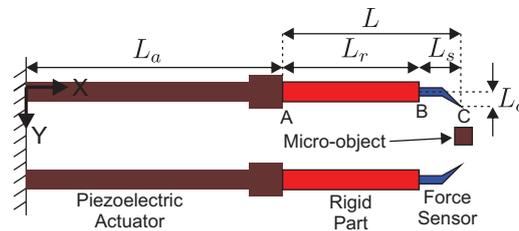
FIGURE 3.14: Complete scheme of the two-smart-fingers microgripper (TSFM).
