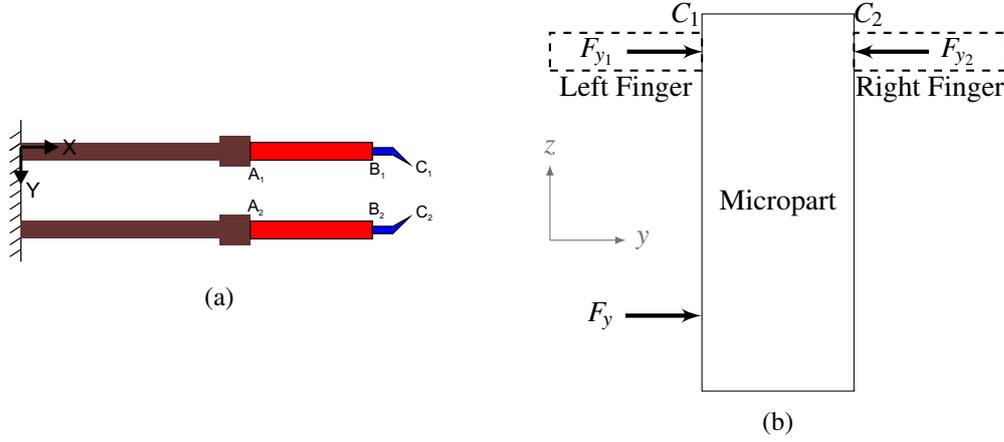
FIGURE 5.6: (a) TSMF initial scheme showing tips A, B and C of the two fingers, (b) a scheme showing the micropart between the fingers of the microgripper and a perturbation force  $F_y$  applied on the micropart,  $F_{y1}$  and  $F_{y2}$  being the gripping forces applied on the micropart.
