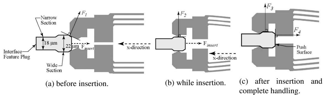
FIGURE 1.12: The handling steps of the micropart using the passive finger [32].
