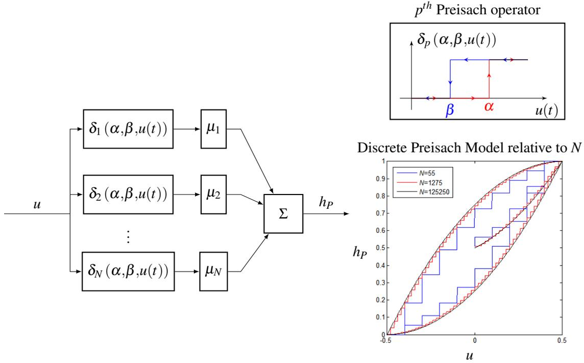
FIGURE 3.7: A block diagram showing the Preisach operators and the output of the hysteresis model,  $h_P$ , as sum of all the Preisach operators with weight functions.
