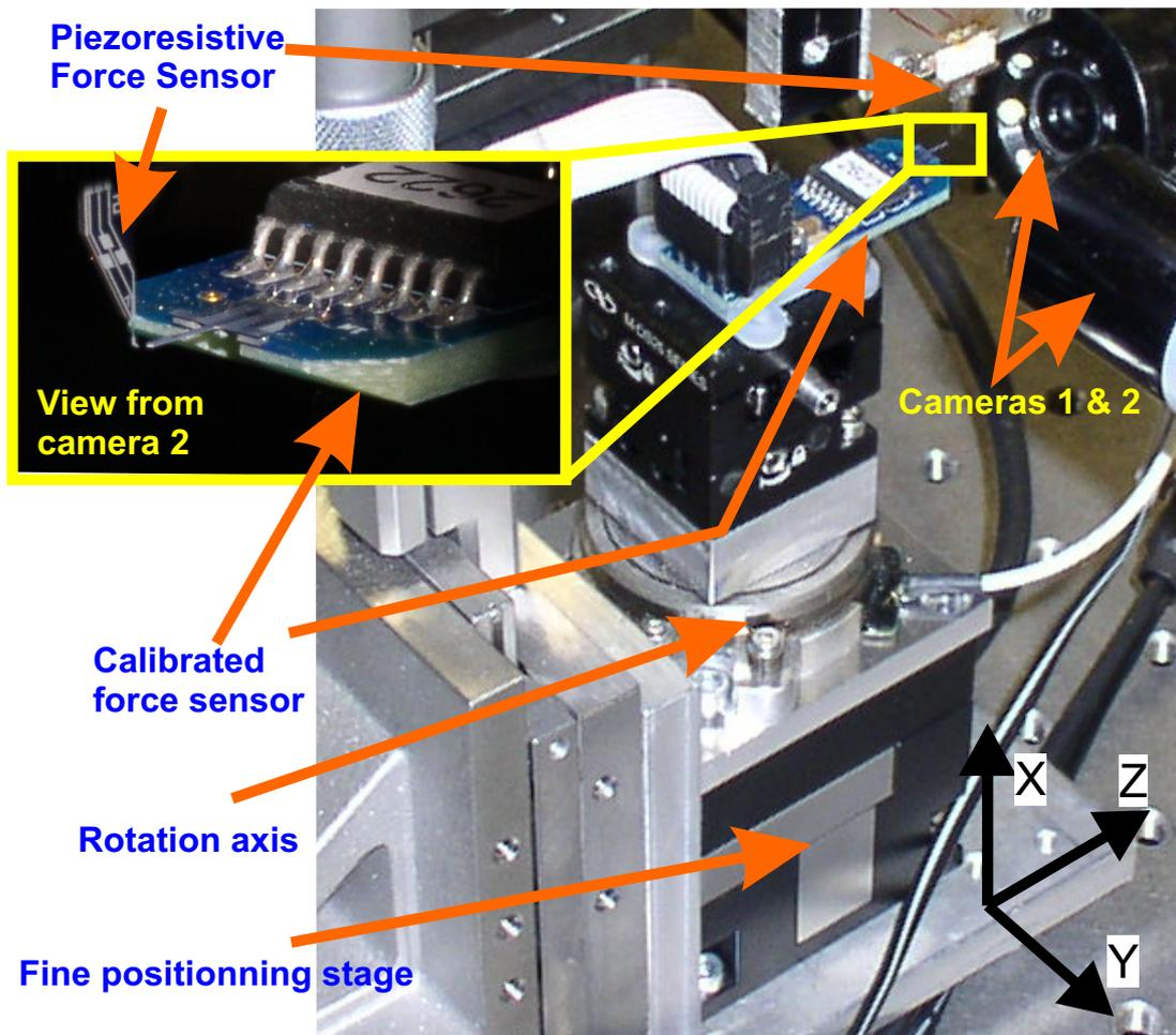
FIGURE 2.11: Experimental setup used for the characterization of the piezoresistive force sensor. A calibrated force sensor (CalibFS) is fixed on a robotic system consisting of a fine positioning stage and rotation stage. The piezoresistive force sensor (PiezoFS) is fixed. Two cameras are used to see the contact.
