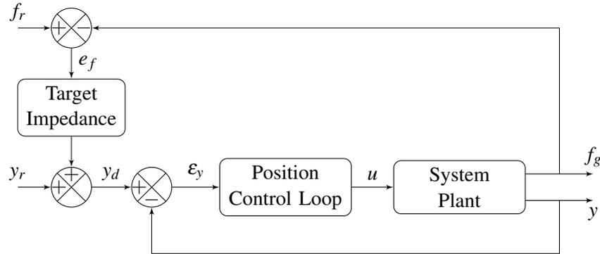
FIGURE 4.6: Position-based impedance control diagram as proposed by [64].
