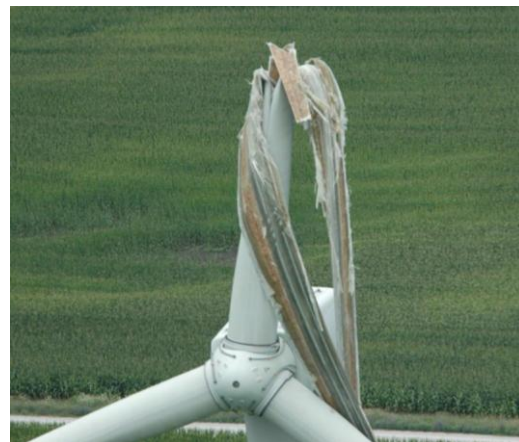
Figure 5: Examples of wind turbine accidents due to blade failures.
