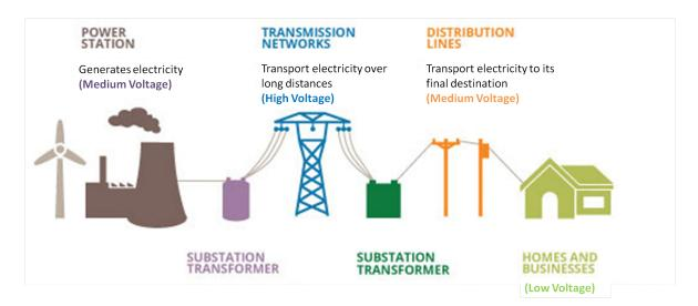
Fig. 1.1: Schematic illustration describing the global network used to the transport of electrical energy. Transmission networks and distribution lines are interconnected through substations transformers.
