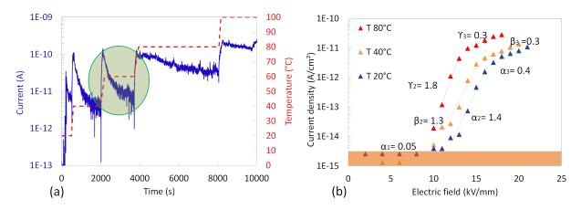
Fig. 2.57: (a) Typical recording of the current for increasing electrode temperature at 12 kV/mm (d = 10 mm) and (b), stabilized current density values for increasing temperatures, in dried  $SF_6$ , at 0.6 MPa, RH = 1.5%.
