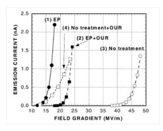
Fig. 2.14: Dark currents versus electrical field for a gap distance of 1 mm, diamond polished electrodes (copper) with various treatments: (1)EP, (2) EP + OUR, (3) no treatment, (4) no treatment +OUR. EP: electro-polishing, OUR: Ozonized Ultra-pure Water Rinsing [18].
