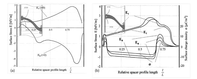
Fig. 1.11: Design shape of insulator used for (a) HVAC GIS and (b) optimized shape withstanding  $750 \, kV$  HVDC, and corresponding electric stress on the insulator surface [30].
