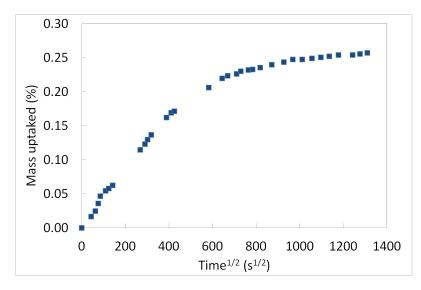
Fig. 3.6: Water absorption measurements of material A on 3.28 mm sample thickness at  $90 \,^{\circ}\text{C}$  and 60% RH.
