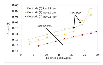
Fig. 2.25: Current measured in  $SF_6$ , versus electric field for three different electrode roughnesses (A), (B) and (C) in negative polarity,  $(0.6 MPa, 20 \,^{\circ}\text{C}, \text{ calculated } RH = 12\%)$ .
