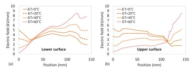
Fig. 4.6: Calculated electric field along the lower (a) and upper (b) surface of the insulator, for different temperature gradient, at  $400 \, kV$ .
