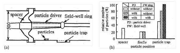
Fig. 1.17: Illustration of a basic insulation structure of a GIS including a particle trap system (a), and experimental results showing the efficiency of a particle driver at DC  $-250 \, kV$ , and with  $3 \, mm$  long aluminum particles (b). [32].
