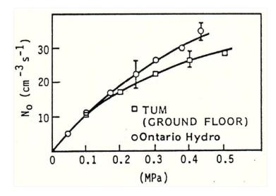
Fig. 2.2: Natural ionization production rates obtained by Munich Technical University and Ontario Hydro, in cylindrical test vessels of differing outer diameters (respectively 52 cm and 27.8 cm diameters) [7].
