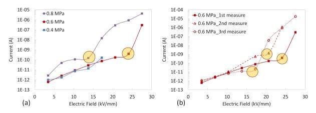
Fig. 2.27: (a) Current measurements in negative polarity depending on electric field with electrode (C) for various pressures. (b) Reproducibility of measurements with 0.6 MPa of  $SF_6$ .
