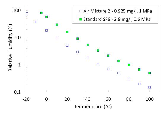
Fig. 18: Example: Variations of relative humidity versus temperature for 1 MPa of air (absolute quantity of water = 0.925 mg/l) and 0.6 MPa of  $SF_6$  (absolute quantity of water = 2.8 mg/l), calculated via the vaisala online calculator (available online: www.vaisala.com).
