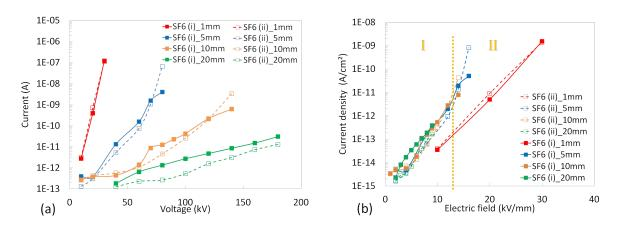
Fig. 2.44: Dark current measurements in standards  $SF_6$  for gap distances from 1 mm up to 20 mm, plotted versus (a) voltage, (b) electric field (0.6 MPa, RH = 20%).
