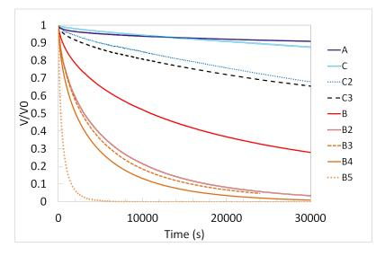
Fig. 3.12: SPD evolution for three epoxy resins and modifications on the catalyst concentration, position and nature, at  $P_1$  (40 °C, RH = 20%).
