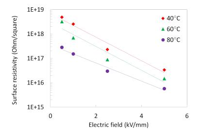
Fig. 3.28: Surface resistivity variations according to electric field and temperature in  $SF_6$  (0.6 MPa), for material A.
