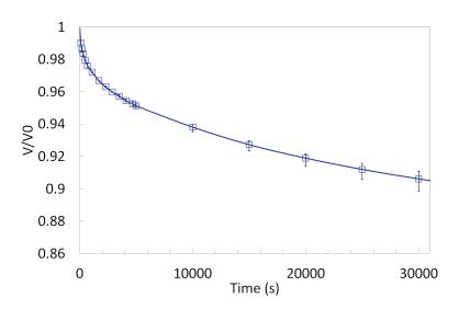
Fig. 3.8: Evaluation of the measurements reproducibility on material A for three dried samples at  $40 \,^{\circ}$ C, RH = 20%.
