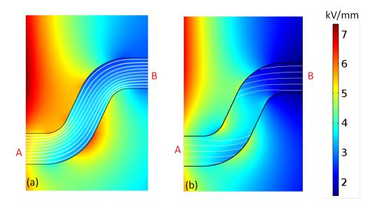
Fig. 4.11: Numerical simulation of the electric field variations (color) and lines of current density (white) without (a) and with (b) implementation of a layer to account for surface properties, at  $20 \,^{\circ}$ C,  $400 \, kV$ .
