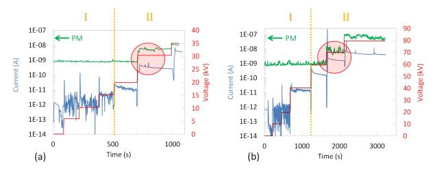
Fig. 2.45: Time-evolution of current and light emission versus voltage in standard  $SF_6$  at 1 MPa for (a) 2 mm gap and (b) 5 mm gap.
