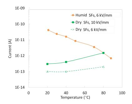
Fig. 2.58: Comparison of currents evolution as a function of electrode temperature in  $SF_6$ , between humid and dry systems at 6 kV/mm and 10 kV/mm (d = 10 mm)
