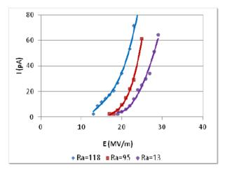
Fig. 2.13: *Dark currents* as a function of field gradient at the cathode surface for a gap distance of 1 mm. *Ra* unit is in nm [15].
