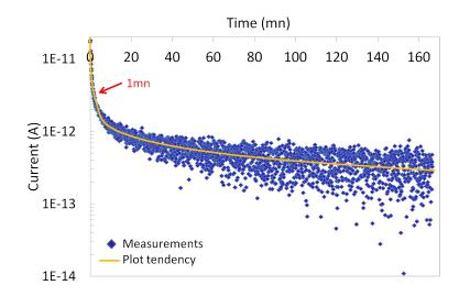
Fig. 3.14: Current measurement versus time. Voltage: 1000 V, at  $40 \degree C$ , RH = 20% on initially dried sample (material A).
