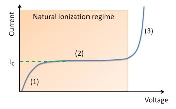
Fig. 2.1: Typical current voltage characteristic for a plane to plane gap in air, (1) and (2) natural ionization regime, (3) corona regime (adapted from [9]).
