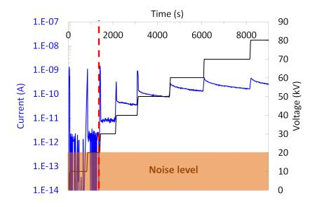
Fig. 2.23: Typical recording of currents versus time and electric field (positive polarity) with brass electrode (B) in  $SF_6$  (0.6 MPa, 20 °C).
