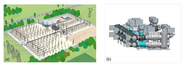
Fig. 1.4: Illustration of (a) an AIS, and (b) a GIS.
