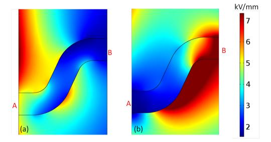
Fig. 4.5: Numerical simulation with (a) an uniform temperature  $T = 20 \,^{\circ}\text{C}$ ; and (b), with a temperature gradient  $\Delta T = 60 \,^{\circ}\text{C}$  ( $V = 400 \, kV$ ).
