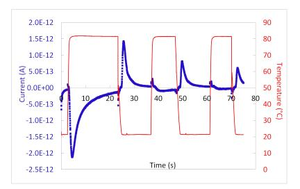
Fig. 3.16: Current measurement versus time and temperature cycling ( $20 \,^{\circ}\text{C} - 80 \,^{\circ}\text{C}$ ) in short-circuit conditions, on material A, under  $SF_6$ .
