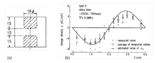
Fig. 1.9: (a) Sectional view of type C insulator, (b) charge distribution after 139 h application of DC voltage [22].
