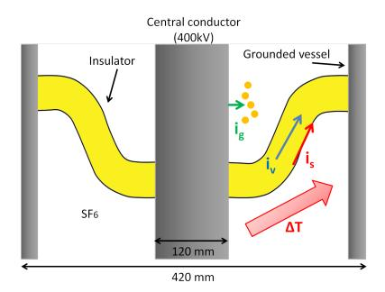
Fig. 4.1: Illustration of the simplified insulator geometry in a GIS structure, and phenomena contributing to electric field distribution and charge accumulation and relaxation.
