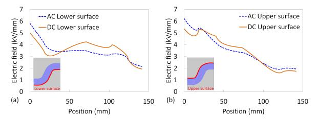
Fig. 4.3: Calculated electric field along (a) the lower and (b), the upper surface of the solid insulator at  $V = 400 \, kV$ ,  $20 \,^{\circ}$ C.
