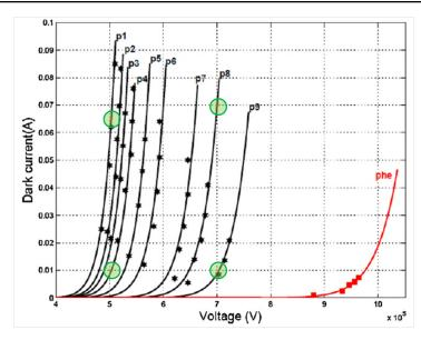
Fig. 2.17: Dependence of the *dark current* as function of the high voltage and pressure (from  $P_1 = 1.7.10^{-3} Pa$  to  $P_9 = 28.2.10^{-3} Pa$ ) in the enclosure. Black lines: Hydrogen gas, red line: Helium gas. [35].
