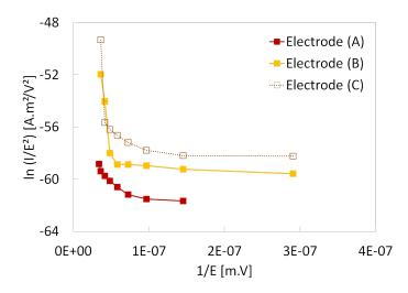
Fig. 2.29: Fowler-Nordheim plots of measured current with different roughnesses in negative polarity (0.6 MPa of  $SF_6$ ,  $20 \,^{\circ}$ C).
