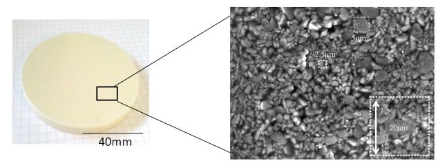
Fig. 3.3: Left: photography of the used sample used. Right: SEM image of the studied material; X2500 - HV20k, SEI.
