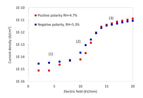
Fig. 2.47: Current density measurements for positive and negative polarities versus electric field, for a gap distance of 10 mm (1 MPa,  $20 \,^{\circ}\text{C}$  and  $RH \simeq 5\%$ ).
