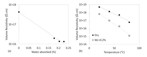
Fig. 3.21: (a) Volume resistivity measurements for various  $W_c$  at 1 kV in air and atmospheric pressure, at T = 60 °C. (b) Volume resistivity versus temperature at 0.2 kV/mm under dry conditions and Wc = 0.2%.  $E_a(dry) = 0.63 eV$ ,  $E_a(0.2\%) = 0.91 eV$ .
