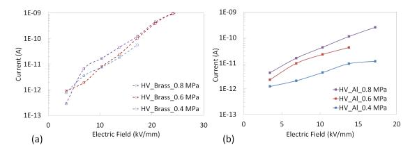
Fig. 2.32: Current measurement in positive polarity in  $SF_6$  for both brass (a), and aluminum (b) HV electrode, depending on the pressure within the enclosure.
