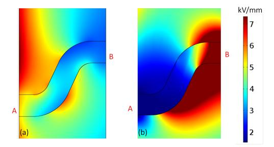
Fig. 4.8: Numerical simulation with (a) an uniform temperature  $T = 20 \,^{\circ}\text{C}$ ; and (b), with a temperature gradient  $\Delta T = 60 \,^{\circ}\text{C}$  ( $V = 400 \, kV$ ), with a water content  $W_c = 0.2\%$ .
