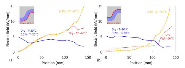
Fig. 4.9: Calculated electric field along the lower (a) and upper (b) surfaces of the insulator, with and without temperature gradient, at  $400 \, kV$ , for both dry and wet materials.
