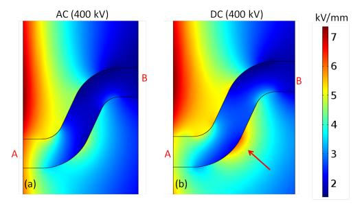
Fig. 4.2: Comparison of electric field intensity (color) in stationary state between AC (a) and DC (b) distribution (axisymmetric calculation of the device presented in figure 4.2,  $V = 400 \, kV$ ,  $20 \,^{\circ}$ C).
