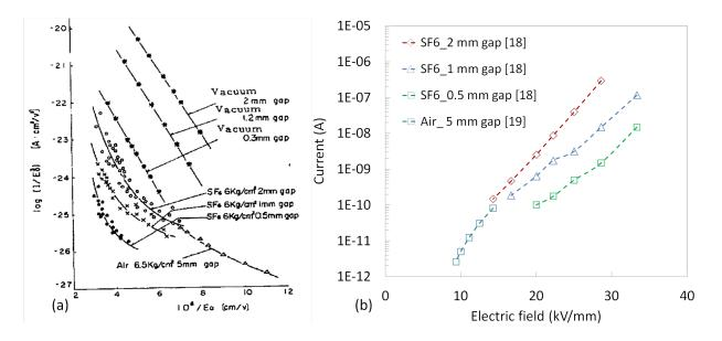
Fig. 2.7: Characteristic of dark current for various gap conditions and nature of gas, with identical electrodes with an area of about  $1 cm^2$ . (a), FN curves, (b), corresponding current versus electric field strength (calculated from (a)) [23].
