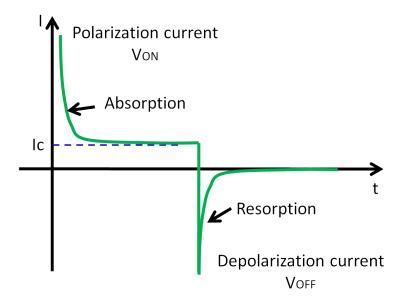
Fig. 3.1: Variations of absorption and resorption current versus time in a solid dielectric during and after electrical stress.
