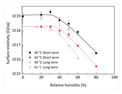
Fig. 3.34: Measurements of surface resistivity versus relative humidity RH and temperature (1 kV).
