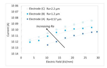
Fig. 2.24: Current measured in  $SF_6$ , versus electric field for three different electrode roughnesses (A), (B) and (C) in positive polarity,  $(0.6 MPa, 20 \,^{\circ}\text{C}, \text{ calculated } RH = 12\%)$ .
