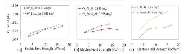
Fig. 2.33: Comparison of current measurements obtained for brass and aluminum electrodes in air mixtures (a) 0.035 mg/l, (b) 0.925 mg/l and (c) 9.26 mg/l.
