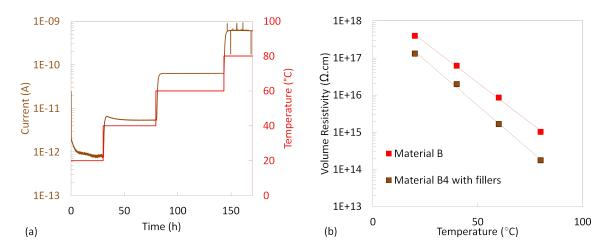
Fig. 3.24: (a) Current measurement on material B4 with fillers at 1000 V and various temperatures. (b) Calculated volume resistivity of B4 with fillers compared to material B, for different temperatures.
