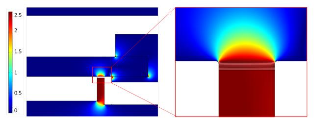
Fig. 3.30: Focus on electric field intensity (color) and lines of current density with a layer added onto the sample surface, between the high voltage and measurement electrode, to account for the electric properties of the insulator surface (axisymmetric calculation,  $\rho_{vL} = 8.10^{15} \Omega.cm$ ,  $\rho_v = 8.33 \cdot 10^{17} \Omega.cm$ ,  $\delta = 320 \,\mu m$ ). Most of current lines flow through the surface layer.
