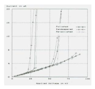
Fig. 2.9: Current measurements depending on electric field strength for a point/plane electrode system at 0.1, 0.3 and 0.6 MPa of  $SF_6$  [21].
