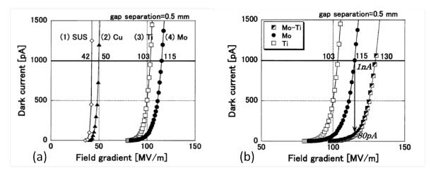
Fig. 2.12: *Dark currents* depending on electric field for (a) four different electrodes: Stainless steel, Copper, Titanium and Molybdenum, for 0.5 mm gap distance; and (b) for three electrodes configurations: *Mo* cathode and *Ti* anode, *Mo* cathode and anode, *Ti* anode and cathode [10].
