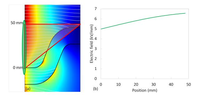
Fig. 4.16: Numerical simulation accounting for both volume and surface properties, with an uniform temperature  $T = 20 \,^{\circ}\text{C}$  at  $400 \, kV$ .
