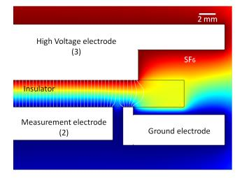
Fig. 3.22: Electric potential intensity (color) and lines of current density corresponding to our experimental setup (axisymmetric calculation of the device presented in figure 3.13, E = 1 kV/mm,  $\rho_v = 2.07.10^{18} \Omega.cm$  at  $20 \,^{\circ}$ C.
