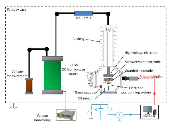
Fig. 2.20: Schema of the experimental test setup built for current measurement through gases under uniform electric field. Maximum voltage: 250 kV.
