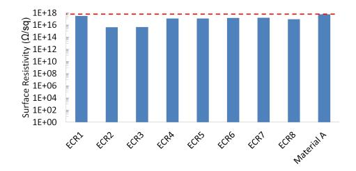
Fig. 3.36: Surface resistivity of ECR1 to ECR8, treated with  $CH_4$  plasma, compared to material A, at 1000 V and  $40 \,^{\circ}$ C.
