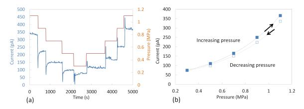
Fig. 2.28: (a),Typical recording of current versus time and pressure in  $SF_6$  with brass electrode (C), at V = 50 kV. And (b), Current measured versus pressure with brass electrode (C) in  $SF_6$  at V = 50 kV.
