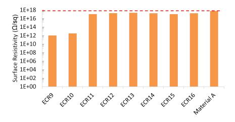
Fig. 3.37: Surface resistivity of ECR9 to ECR16, treated with argon plasma, compared to material A, at 1000 V and  $40 \,^{\circ}$ C.
