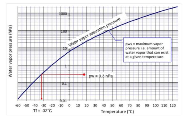
Fig. 17: Example: water vapor pressure 0.3 hPa versus dew point. (available online: www.vaisala.com)
