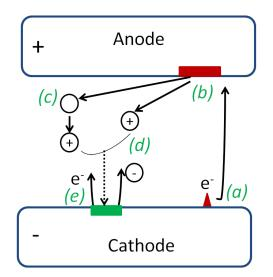
Fig. 2.4: Schematic presentation of primary and secondary emission by bombardment [10].
