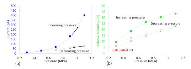
Fig. 2.34: (a) Current measurements performed with brass electrode (C) in  $SF_6$ , versus pressure (50 kV, 20 °C). (b), RH measurements performed in  $SF_6$ , versus pressure, corresponding to (a).
