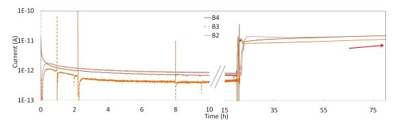
Fig. 3.23: Typical recording of current through materials B2, B3 and B4 at 1000 V and for  $20 \,^{\circ}\text{C}$  (on the left) and  $40 \,^{\circ}\text{C}$  (on the right).
