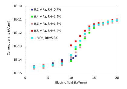
Fig. 2.51: Measured current density for different pressures, in dried  $SF_6$ , at d = 10 mm (20 °C).
