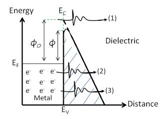
Fig. 2.5: Band diagram at the metal-dielectric interface. (1) *Schottky* emission, (2) Tunnel effect after a gain in energy, (3) Tunnel effect for a constant energy.  $E_v$  and  $E_c$  representing respectively the energy corresponding to the higher level of the valence band, and the lower level of the conduction band.
