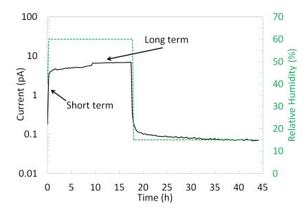
Fig. 3.33: Variations of the recorded current when the relative humidity RH is varied between 15 and 60% (1 kV, 60 °C).
