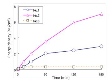
Fig. 1.15: Measurements of charge density over time for three different spacer surface and electrode conditions presented in table 1.1 [21].
