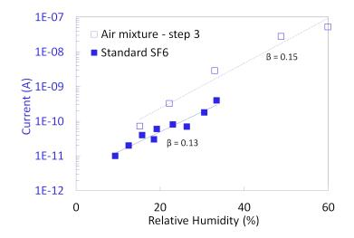
Fig. 2.43: Current measurements depending on relative humidity in air at different temperatures (step 3 at 35 kV) and in  $SF_6$  at different pressures (at 50 kV), with  $\alpha$  the corresponding slopes.
