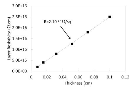
Fig. 3.31: Layer resistivity  $\rho_{vL}$  providing a good agreement between measured and calculated currents, versus arbitrary layer thickness  $\delta$ .  $V = 5 \, kV$ ,  $\rho_v = 8.33.10^{17} \Omega.cm$ ,  $\rho_g = 1.10^{25} \Omega.cm$ ,  $40 \,^{\circ}$ C.
