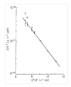
Fig. 2.10: FN for current measured in air depending on electric field strength for a plane to plane electrode system [24].
