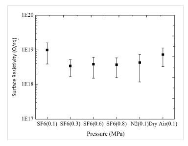
Fig. 3.27: Surface resistivity evolution with gas nature and pressure in  $SF_6$  in dry conditions (dried sample,  $40 \,^{\circ}\text{C}$ ,  $0.5 \, kV/mm$ ).
