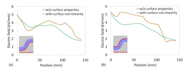
Fig. 4.12: Calculated electric field along the lower (a) and upper (b) surfaces of the insulator at  $20 \,^{\circ}$ C,  $400 \, kV$ .
