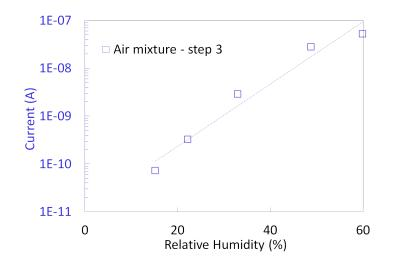
Fig. 2.39: Current measurements performed with electrode (C) in step 3, versus relative humidity, at 35 kV.
