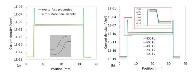
Fig. 4.13: Calculated current density along a section of the insulator at  $20 \,^{\circ}$ C, showing (a) the current density through the insulator volume and its surface layer at  $400 \, kV$ , and (b) the variations of current density for various voltages.
