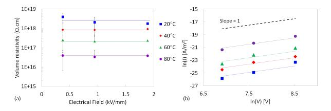
Fig. 3.18: (a) Volume resistivity variations according to electric field and temperature in  $SF_6$  (0.5 MPa), (b) SCLC representation, for material A.
