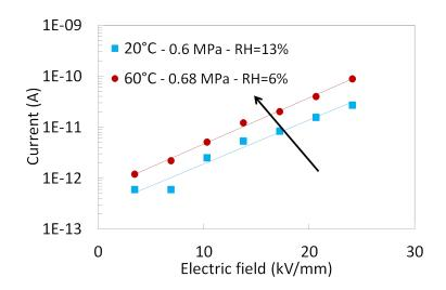
Fig. 2.40: Current variations in case of  $SF_6$  with RH = 13% at  $20 \,^{\circ}\text{C}$  and  $0.6 \, MPa$ , with increasing temperatures.
