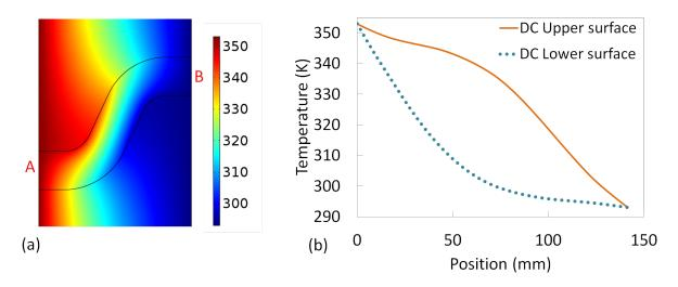
Fig. 4.4: (a) Temperature gradient within the insulator when the conductor (A) is at  $80 \,^{\circ}\text{C}$  and the grounded vessel (B) at  $20 \,^{\circ}\text{C}$ . (b) Repartition of the temperature from the conductor ( $x = 0 \, mm$ ) toward the vessel ( $x = 145 \, mm$ ) on the lower and upper surface of the solid insulator.
