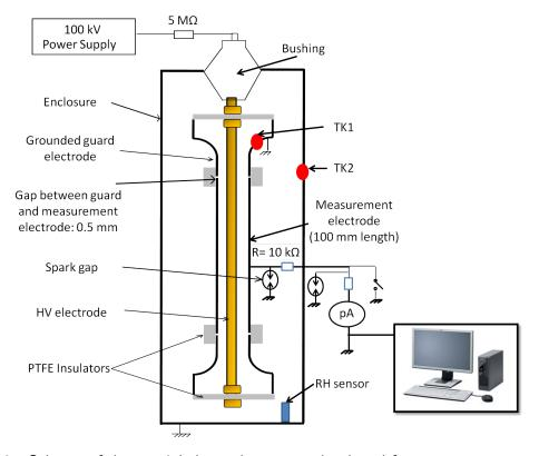
Fig. 2.18: Schema of the coaxial electrodes system developed for current measurements. (Maximum voltage:  $100 \, kV$ )
