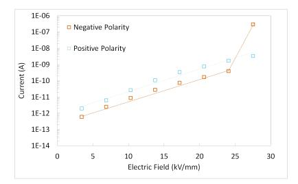
Fig. 2.26: Comparison of measured current in positive and negative polarity in  $SF_6$ , in case of electrode (C) (0.6 MPa,  $20 \,^{\circ}$ C, calculated RH = 12%).
