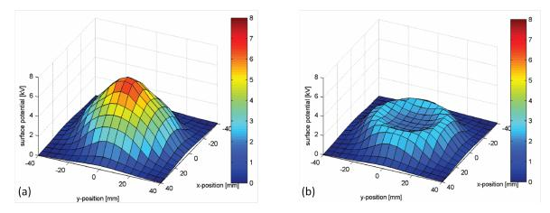
Fig. 1.19: Surface potential distribution on epoxy resin (a) immediately after charge deposition, (b) after  $660 \min [49]$ .
