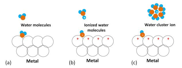
Fig. 2.61: Representation of mechanism proposed for water ion cluster formation, adapted from [43]. (a) Water molecule adsorbed on metal surface, (b) ionization of water molecule due to field desorption mechanism and (c), creation of a water cluster ion.
