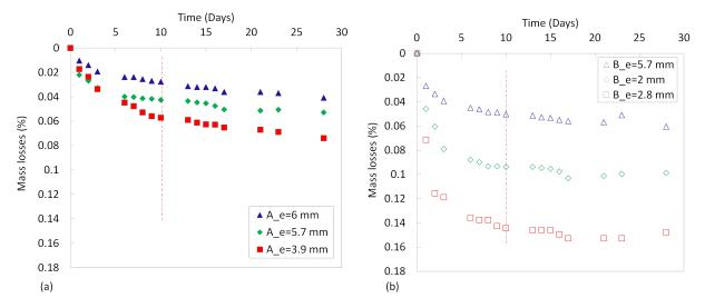
Fig. 3.4: Determination of the drying time in the vacuum oven at  $65 \,^{\circ}\text{C}$  for both material A (a), and B (b).
