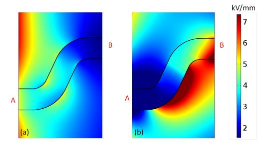
Fig. 4.14: Numerical simulation with (a) an uniform temperature  $T = 20 \,^{\circ}\text{C}$ ; and (b), with a temperature gradient  $\Delta T = 60 \,^{\circ}\text{C}$  at  $400 \, kV$ .
