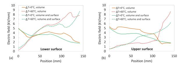
Fig. 4.15: Calculated electric field for both simulation models: neglecting or not the surface properties, in presence of a temperature gradient, at 400 kV for (a) lower and (b) upper surfaces.
