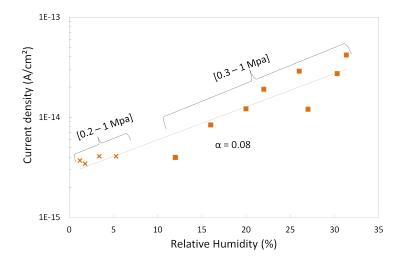
Fig. 2.53: Current measurements depending on relative humidity in  $SF_6$  (at 6 kV/mm, 20 °C).
