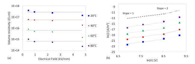
Fig. 3.19: (a) Volume resistivity variations according to electric field and temperature in  $SF_6$  (0.6 MPa), (b) SCLC representation, for material B.
