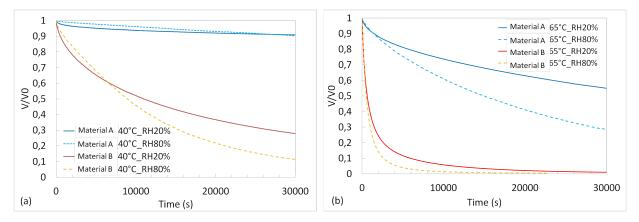
Fig. 3.9: SPD evolution on material A and B at (a)  $40 \degree C$  ( $P_1$  and  $P_2$ ) and (b)  $65 \degree C$  ( $P_3$  and  $P_4$ ).
