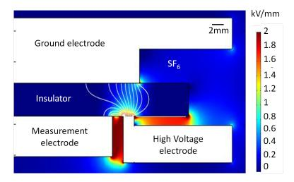
Fig. 3.29: Electric field intensity (color) and lines of current density corresponding to our experimental setup (axisymmetric calculation of the device presented in figure 3.25, V = 5 kV,  $\rho_v = 8.33 \cdot 10^{17} \Omega.cm$ ,  $\rho_g = 1.10^{25} \Omega.cm$ ,  $40 \,^{\circ}\text{C}$ .
