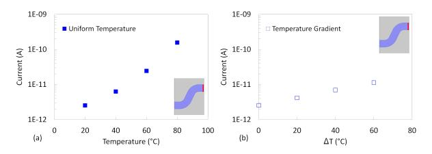
Fig. 4.7: Calculated current through the solid insulator in case of uniform temperatures (a) and temperature gradients (b), at  $400 \, kV$ .
