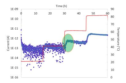
Fig. 3.17: Typical recording of current on material A under 1 kV/mm in 0.5 MPa of  $SF_6$ , for different temperatures.
