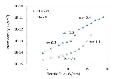
Fig. 2.52: Measured current density for two different RH, corresponding to conditioning  $C_1$  and  $C_2$ , in  $SF_6$  at 0.6 MPa.
