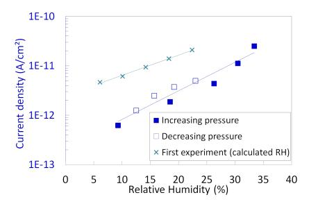
Fig. 2.35: Current measurements performed with brass electrode (C) in  $SF_6$ , versus relative humidity (50 kV, 20 °C) with calculated and measured RH values.
