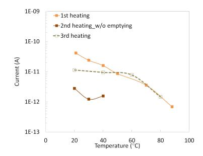
Fig. 2.56: Three series of stabilized current measurements for increasing temperature, at +70 kV, 1 MPa of  $SF_6$  with RH = 20%.
