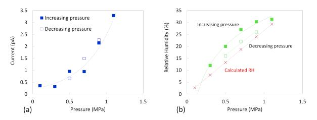
Fig. 2.49: (a) Current and (b) RH measurements performed in  $SF_6$ , with pressure variations (60 kV,  $20 \,^{\circ}$ C).
