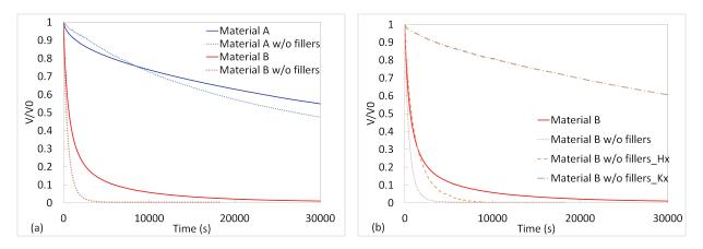
Fig. 3.11: SPD variations for (a) both materials A and B, with and without fillers, and (b) material B with various chemical compositions ( $H_x$ : other hardener,  $K_x$  other catalyst), at 65 °C, RH = 20%.
