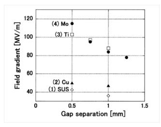
Fig. 2.16: Gap separation dependence of the field, corresponding to a *dark current* of 1 nA for four electrodes: Stainless steel, Titanium, Copper and Molybdenum [10].
