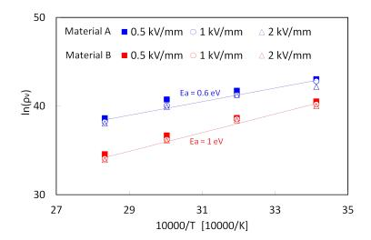
Fig. 3.20: Arrhenius plot showing the thermal evolution of volume resistivity for both material A and B.
