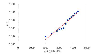
Fig. 2.60: Representation of the measured current in  $ln(J) = f(E^{1/2})$ .
