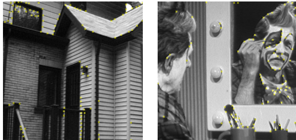
Figure 12. Salient points (isolated points in the feature space back-projected in the image): 100 rarest pixels ( m = 10 , Local jet of order 2, one single scale \sigma = 1.5 , no quantisation); a minimal exclusion distance of 5 pixels is used to avoid clustering of the salient pixels.
