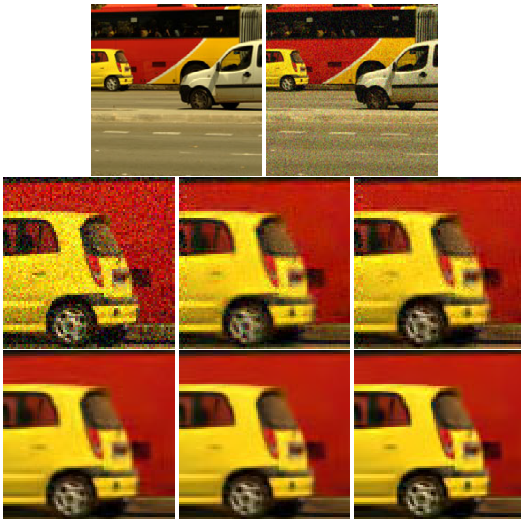
Figure 3.1: Top: original and noisy images with an additive Gaussian white noise of standard deviation 25. Below, from top to bottom and left to right: crop of denoised images by sliding DCT thresholding filter and incrementally adding use of a Y_oU_oV_o colour system, uniform aggregation, variance based aggregation and iteration with the “oracle” given by the first step. The corresponding PSNR are 26.85, 27.33, 30.65, 30.73, 31.25.
