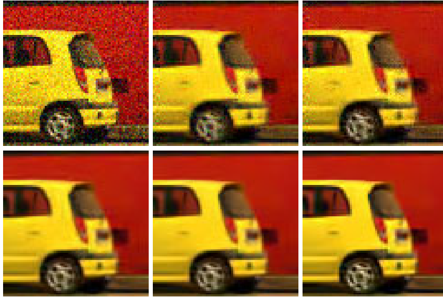
Figure 1: From top to bottom and left to right: crop of the noisy input image ( \sigma = 25 ), and denoised images by sliding DCT thresholding filter and incrementally adding use of a Y_oU_oV_o colour system, uniform aggregation, variance based aggregation and iteration with the “oracle” given by the first step. The corresponding PSNR are 26.85, 27.33, 30.65, 30.73, 31.25.
