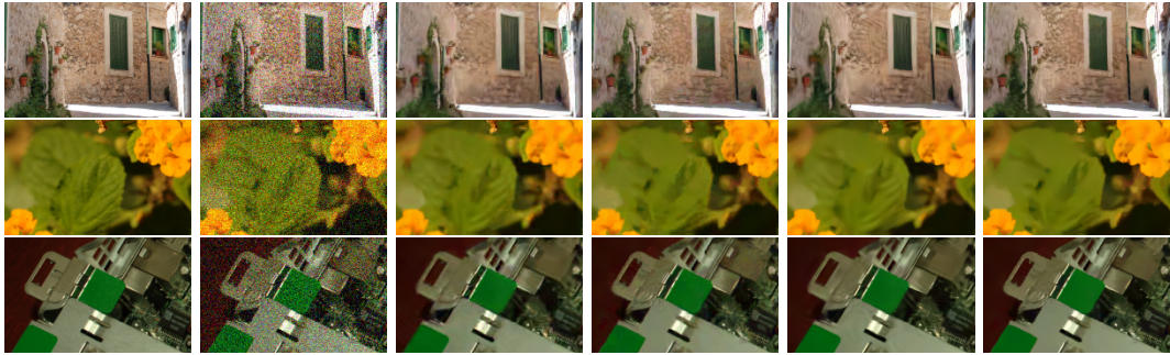
Figure 4.9: Crops from the results of the images Alley, Flowers and Computer. From left to right: the original image, the noisy image ( \sigma = 30 ), the outputs of BM3D, NL-Bayes, DDID, and NLDD. Full results are available in the article’s website.
