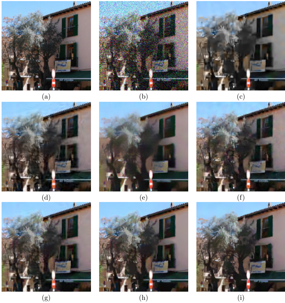
Figure 5.7: Comparison of visual quality. The noisy image was obtained adding a Gaussian white noise of standard deviation 40. From top to bottom and left to right: original, noisy, DCT sliding window, BLS-GSM, NL-means, K-SVD, BM3D, Non-local Bayes and NLDD.
