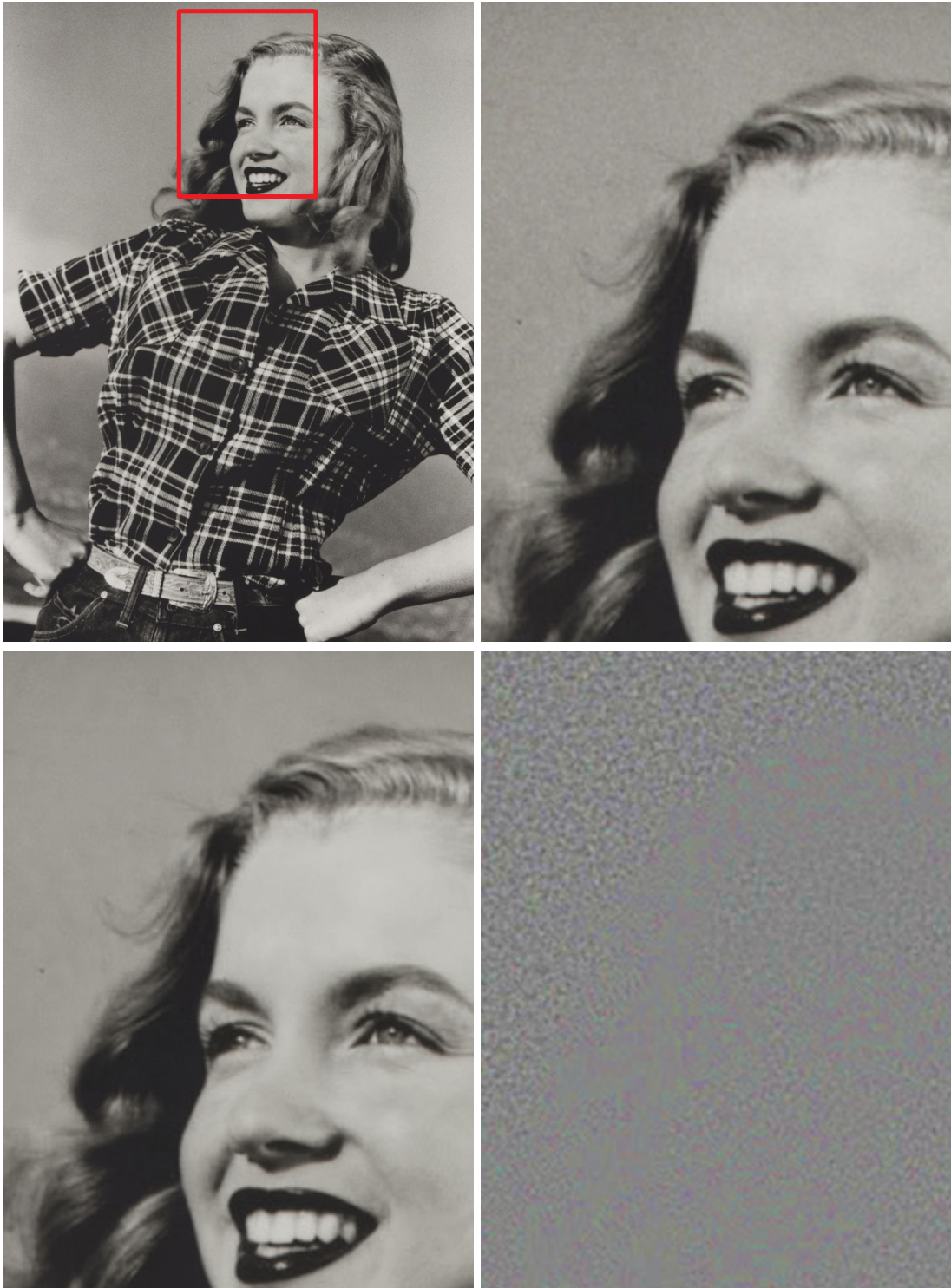
Figure 9.22: Blind denoising on “Marilyn”, using two scales. From left to right, top to bottom : input noisy image, crop of the noisy image, crop of the output denoised image, crop of the difference image.
