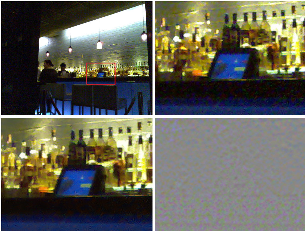
Figure 9.20: Blind denoising on “Bar”, using three scales. From left to right, top to bottom : input noisy image, crop of the noisy image, crop of the output denoised image, crop of the difference image.
