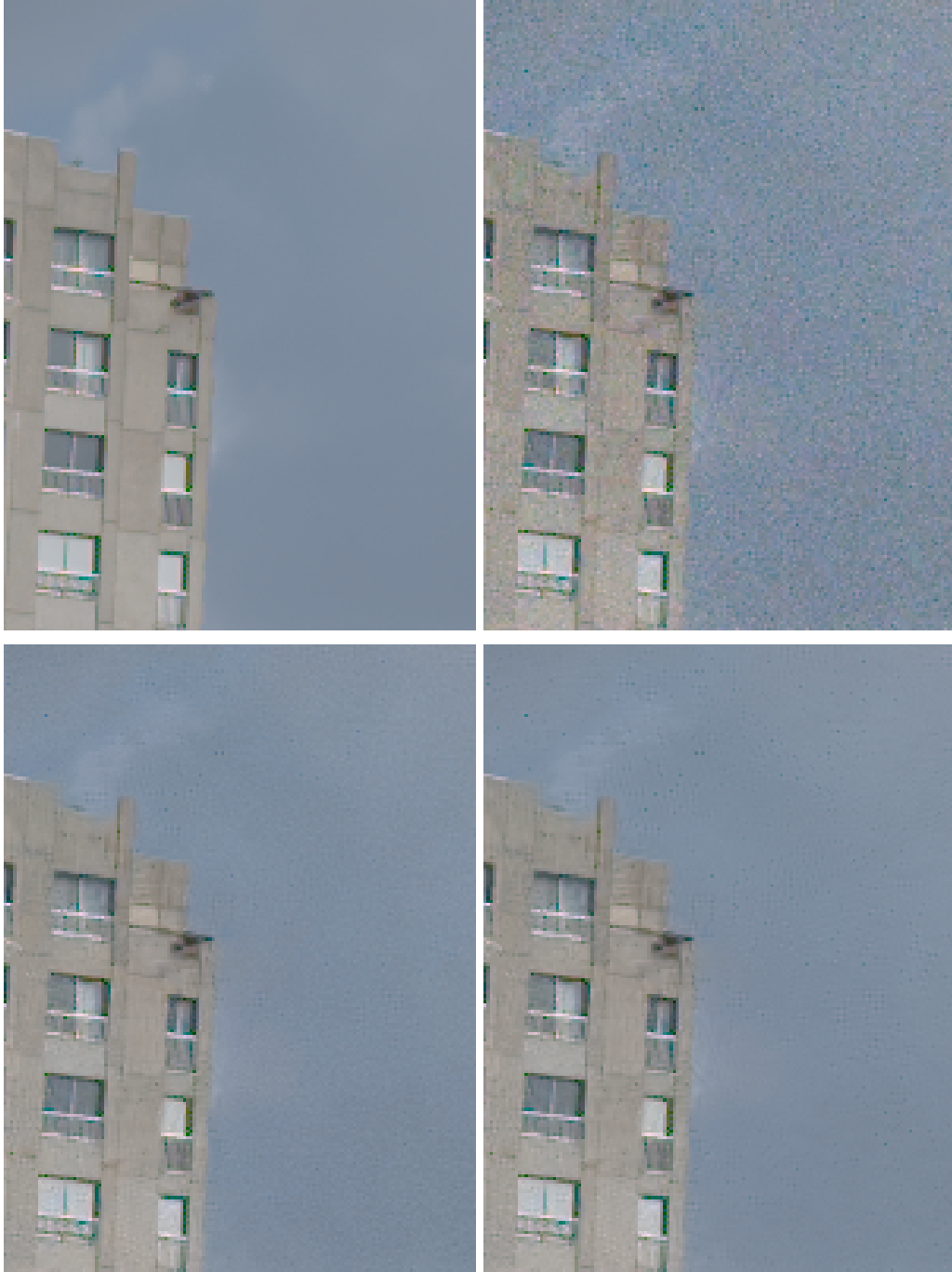
Figure 9.9: Visual results of the demosaicking (second) experiment. From top to bottom, and left to right: crop of the noise-free image u_d , crop of the noisy image \tilde{u}_d , crop of the result of the Noise Clinic using two scales \hat{u}_d|^{s_2} and crop of the result of the Noise Clinic using three scales \hat{u}_d|^{s_3} .
