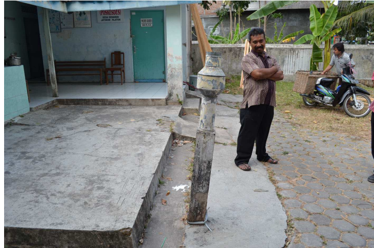
Figure 3.2: Deficient raingauge at Gedaren village.
