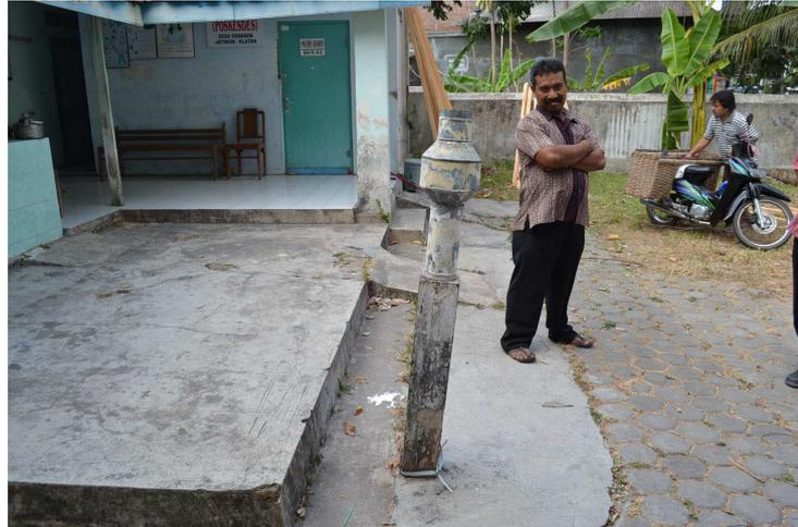
Figure 3.2: Deficient raingauge at Gedaren village.
