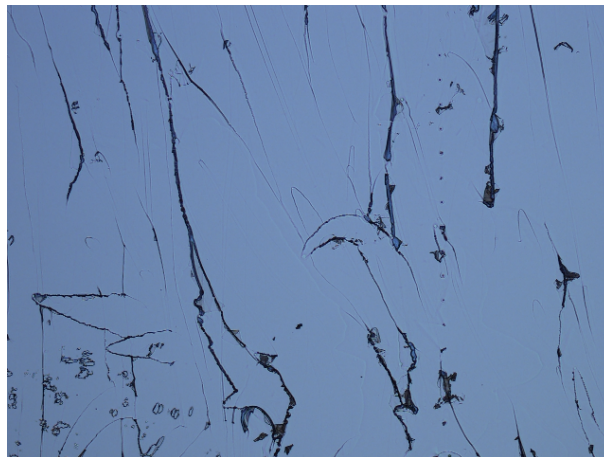
Figure 3.12: Optical microscope picture of a broken oxide film on a processed sample surface, resulting from a too short under-etching time.
