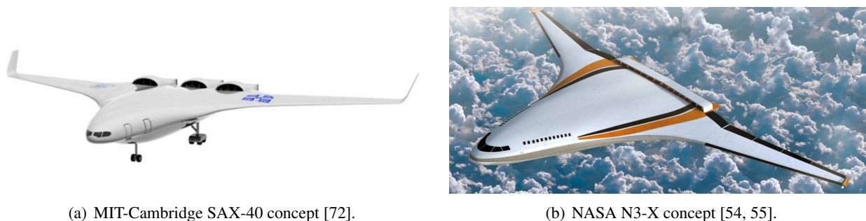
Figure 4-24: Typical studies of Blended Wing-Body (BWB) configurations with Boundary Layer Ingestion (BLI).
