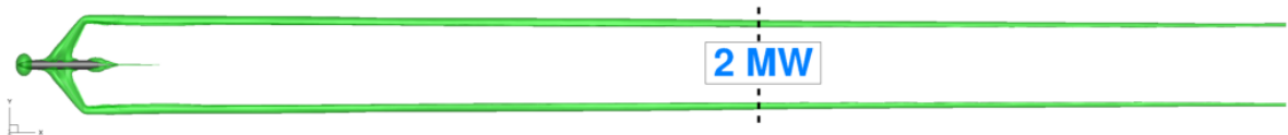
Figure 3-43: Isosurface of transverse kinetic energy ( v^2 + w^2 ) and work potential evaluated 70 mean aerodynamic chords. Super-fine mesh (L6).
