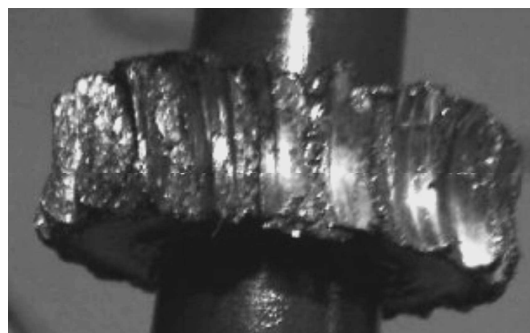
Figure 8 – Abrasive wear of a worm gear
