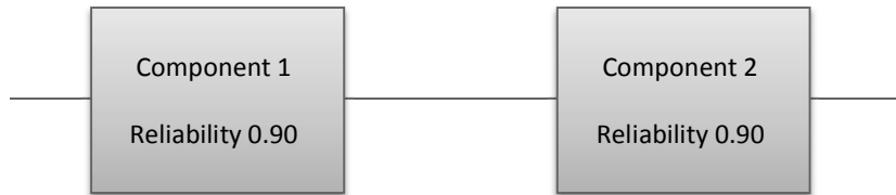
Figure 19 – Reliability block diagram of 2 components in series
