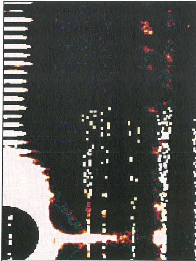
Fig. III.10 : The Kajava unit cell predicts additional row-lines in the central region of collagen X-ray pattern. Thus, following a subtraction of background from all the images in the same pack and image addition to improve the weakest intensity peaks I show here the overlap of predicted and experimental data. The Kajava model obviously doesn't fit the experimental pattern since no additional row-lines are observed in the central region. The conventional experimental row-lines are here clearly identified but the position and the split of the (-1,0,l) and (1,0,l) row-lines is also not followed by the new model.
