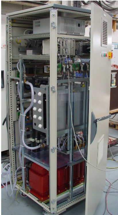
Fig. 2: Current Active Load (CAL) in test
