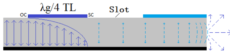
Figure 2.35: Illustration of side radiation (dashed) and RF power suppression (solid).
