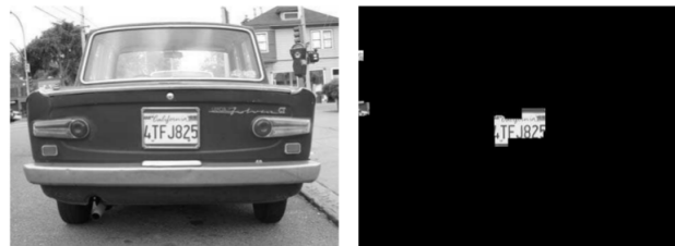
Figure 4.9 – Vehicle registration plate input and output images
