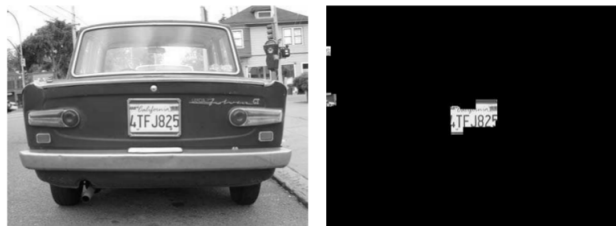
Figure 4.9 – Vehicle registration plate input and output images
