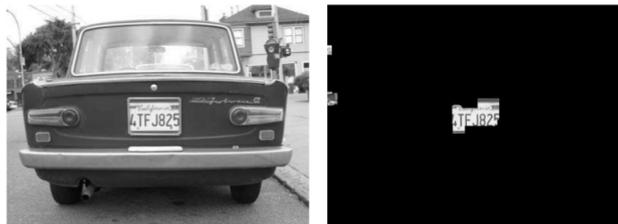
Figure 4.9 – Vehicle registration plate input and output images
