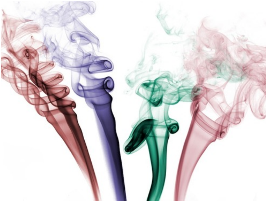
Figure 1.1: Buoyant plumes of smoke. Their visualization demonstrates three types of fluid flow: laminar , transitional , and turbulent . At the bottom of the photo, the plumes are smooth and orderly, as is typical for laminar flow . Despite the quiescent air, tiny perturbations sneak into the flow causing periodical vortical whorls, as we can observe mostly on the first plume; the flow is in transition . Then, disturbances in the plume get amplified and break down into turbulence ; near the top of the image, we observe the smoke's movement: chaotic and intermittent, full of turbulent eddies. (Photo credit: Gizmodo Shooting Challenge )
