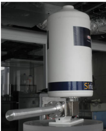
Figure 3.6: Picture of one Si(Li) detector connected to its liquid nitrogen cryostat.
