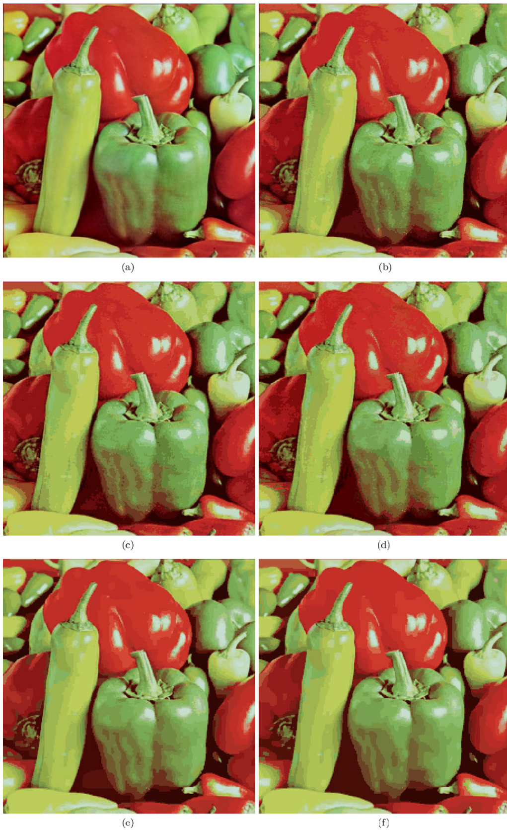
Fig. 4 (a) is the original image, (b, c, d) the Wu, K-means and median-cut results respectively; (e, f) show our result for \mu equal 25 and 50 respectively. Note that there are many isolated small regions in (b, c, d), while both (e) and (f) feature only smooth large regions, retaining global aspect nonetheless
