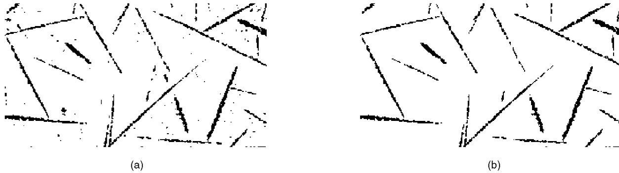
Fig. 9. Filtering of images of fibers corrupted by electronic noise due to the acquisition device (microprobe). A union of directional rank-max openings removes the noise and preserves most fibers. (a) 295 \times 164 image f of fibers. (b) Output image: \bigvee_{\theta} \gamma_{L_{151, \theta, 11}}(f) .
