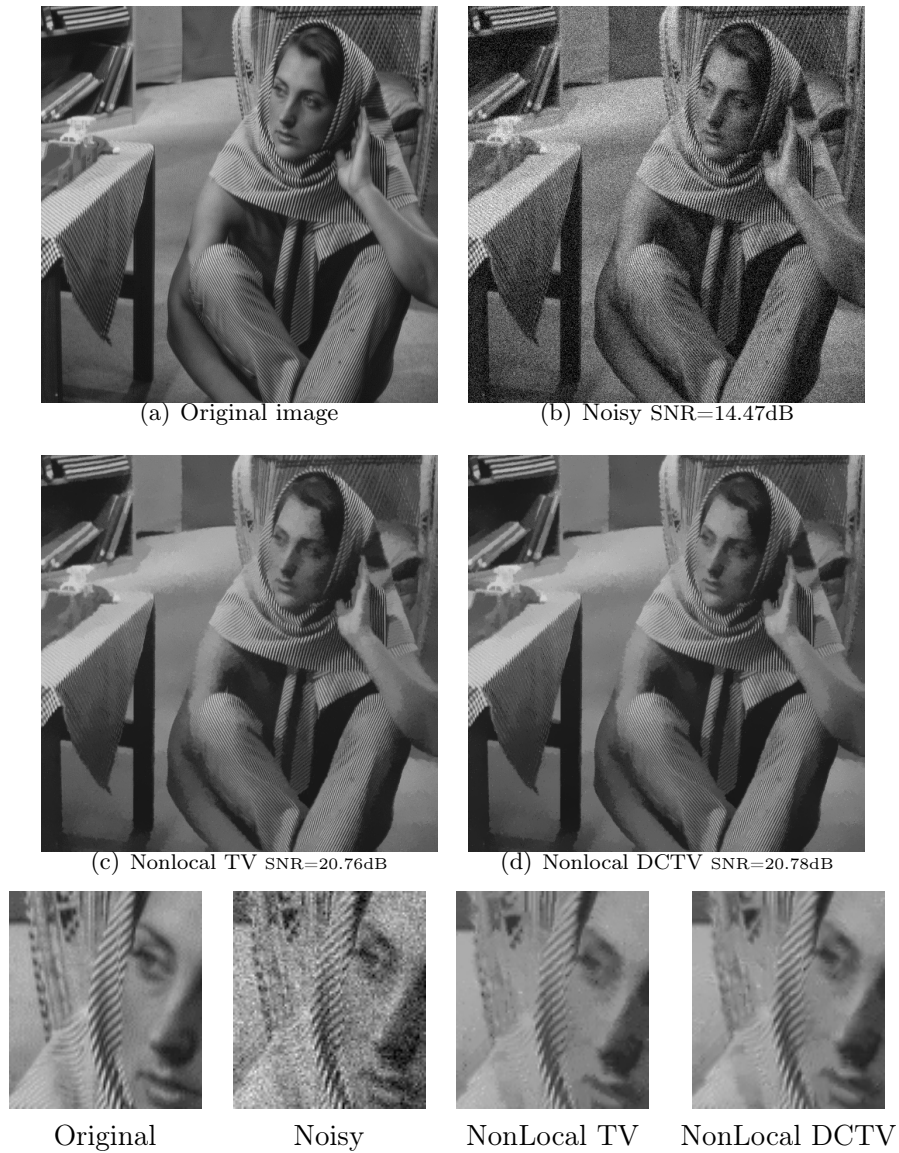
Figure 5.7: Local and nonlocal denoising (Gaussian noise of variance \sigma^2 = 20 ). The nonlocal weights are computed using Bresson (2009). Regularization parameters used to obtain the best results: (e) \lambda = 0.048 (f) \lambda = 0.093 .
