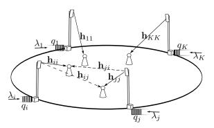
Figure 3.1: Illustration of the system model of the interference channel with queues at the transmitters
