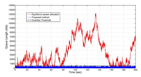
Figure 3.3: Evolution of the queue lengths at transmitter 1 in the three-links setting in one simulation run, using the equilibrium and the proposed power allocation method.
