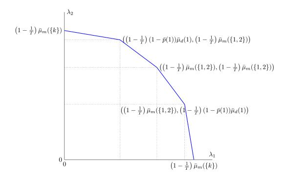
Figure 4.6: Stability region of the mixed policy for a system with 2 users with i.i.d. channels and single rate level.
