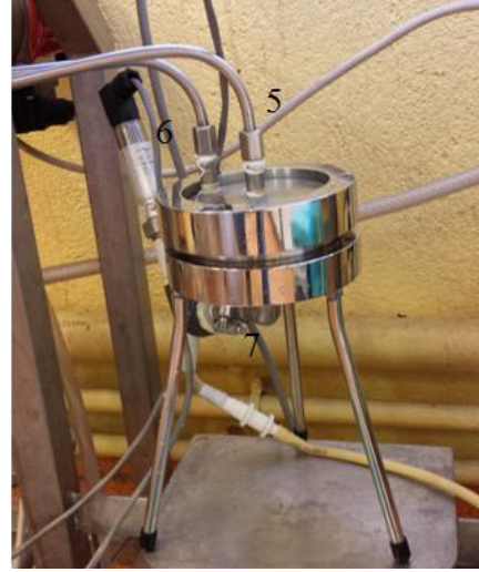
Figure III. 5: Cellule de filtration tangentielle (membrane plane)
