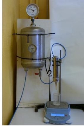
Figure III. 9: Pilote de filtration frontale
