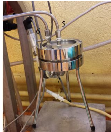
Figure III. 5: Cellule de filtration tangentielle (membrane plane)
