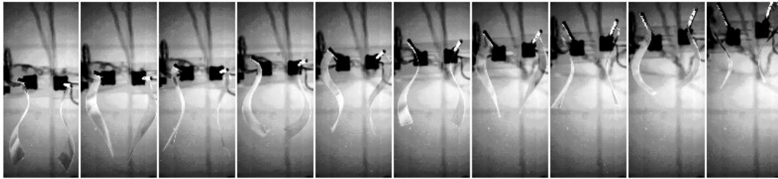
Figure 6.4: Two self-propelled swimmers in a side-by-side configuration. Each foil is held by an independent air-bearing rail. In the image sequence presented the two foils are actuated in anti-phase.
