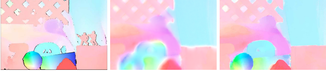
Fig. 2.8: Comparison of regularization strategies using the Army optical flow dataset by Baker et al. (2007) . From left to right: (a) ground truth of the motion, (b) motion estimate using l_2 -regularization ( Horn and Schunck, 1981 ), and (c) motion estimate using TV-regularization ( Wedel et al., 2009 ). Unlike l_2 -regularization that over-smooths the solution because its quadratic penalty, TV respects motion discontinuities thanks to its l_1 -based penalty. (Images courtesy of Mark Werlberger)
