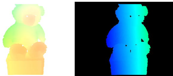
Fig. 6.24: Results of the rigid motion experiment. From left to right: (a) optical flow and (b) Z -component of the scene flow, respectively.
