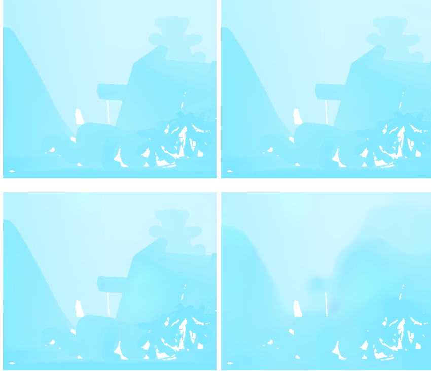
Fig. 6.4: Optical flow estimates for the Teddy stereo dataset. From left to right, from top to bottom: (a) Ground-truth, and (b) twist-motion, (c) 3D-motion and (d) 2D-motion representations.
