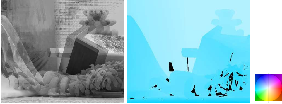
Fig. 6.2: Optical flow for the Teddy dataset. From left to right: (a) Blend of first and second brightness images, (b) ground truth of the optical flow, and (c) optical flow color coding. Observe that every pixel performs a purely horizontal motion, whose magnitude is a function of its depth.
